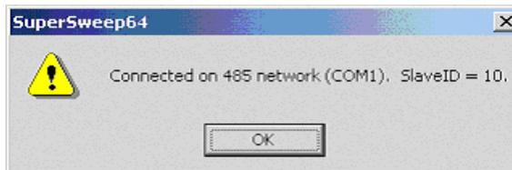
**Figure 3-11. Serial Connection Confirmation**
