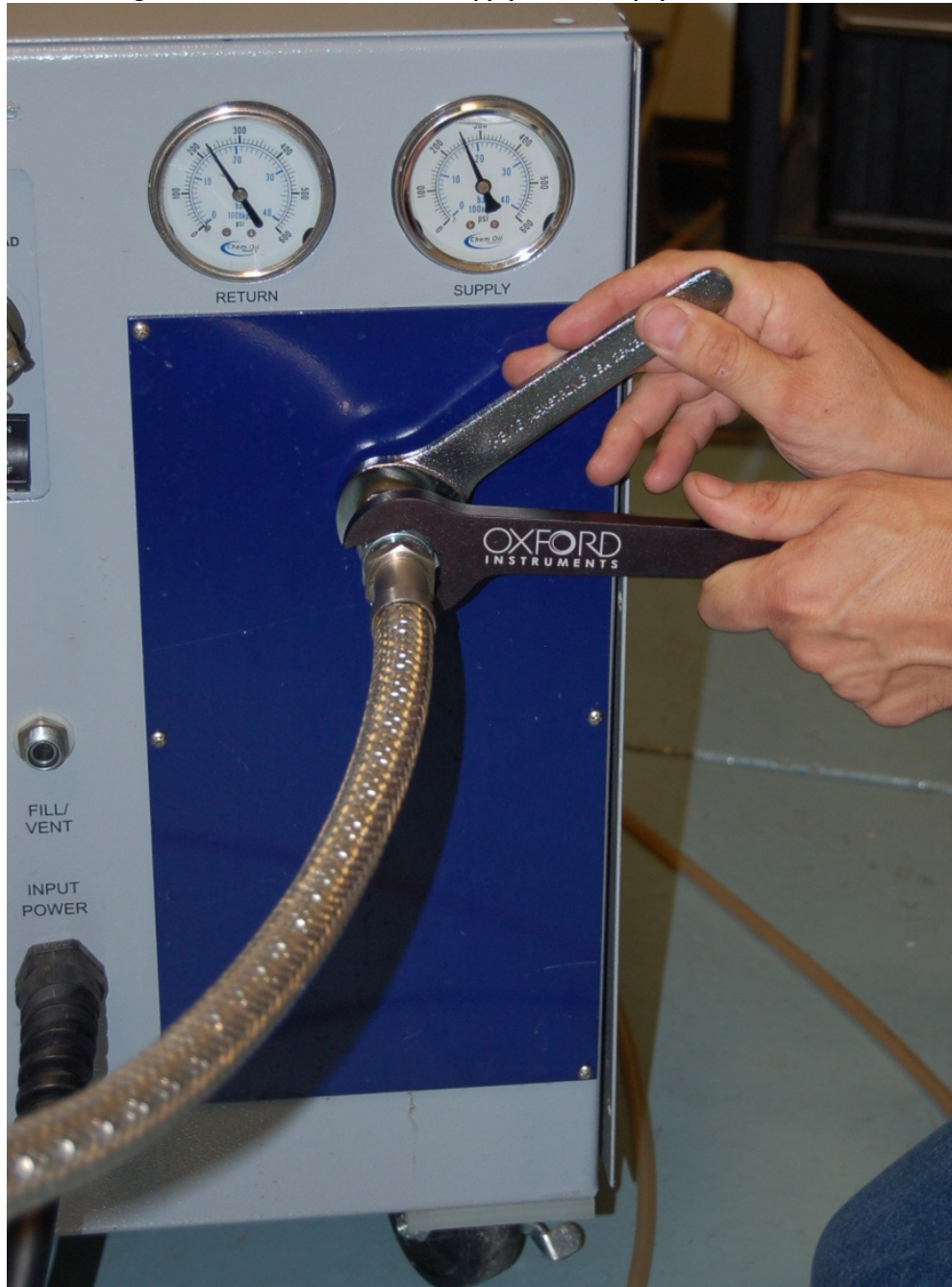
Figure 13 – Removal of Helium Supply Line Aeroquip at Access Panel
