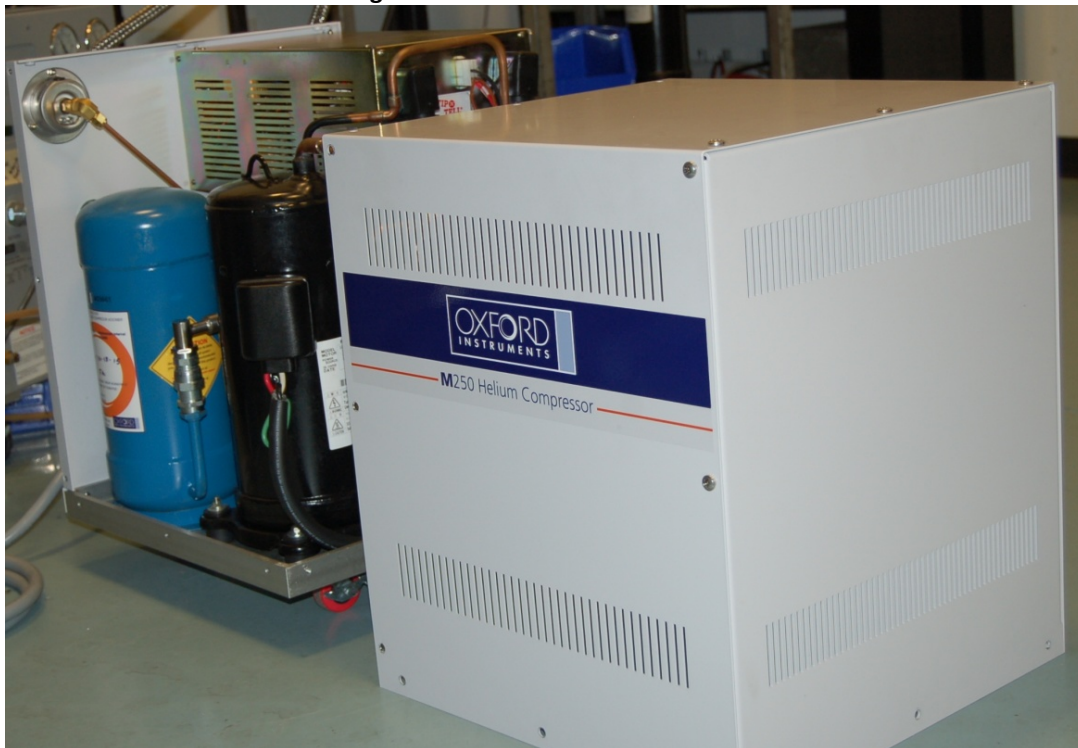
Figure 6 – Removal of Cover Panels
