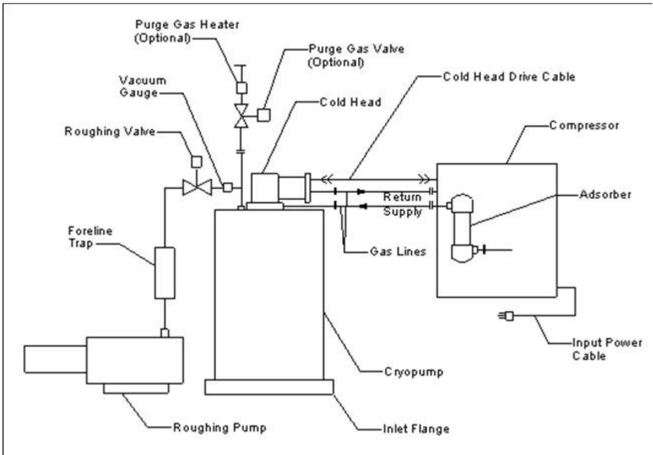
Figure 3 – Connection Diagram
