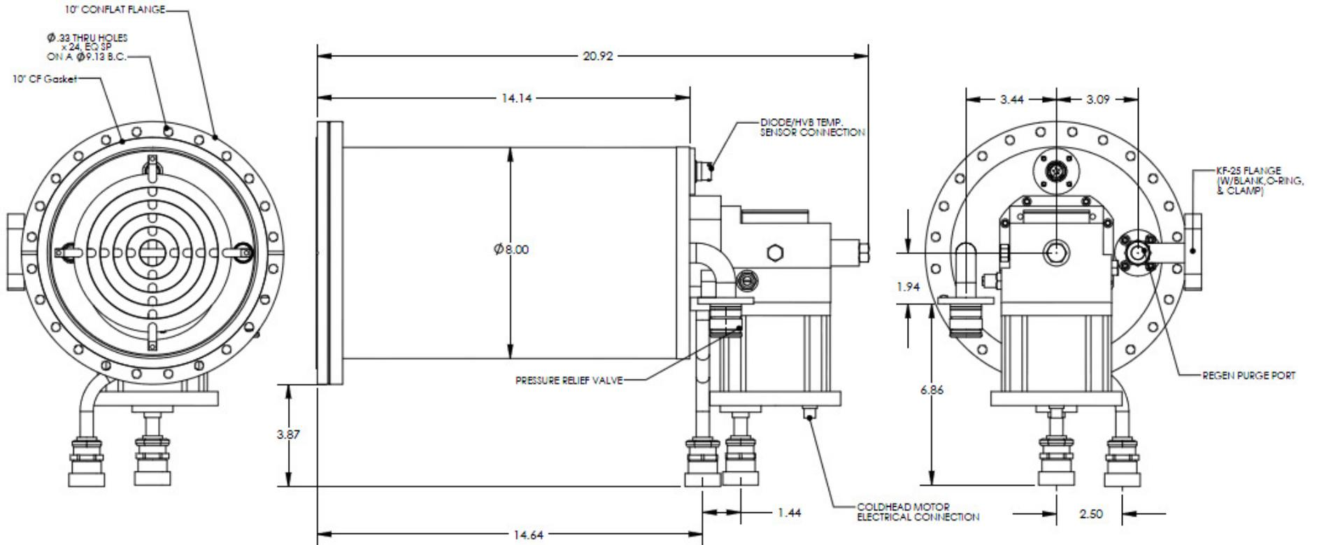
Figure 1 – Cryo-Plex 8 Cryopump with CF Inlet Dimensions
