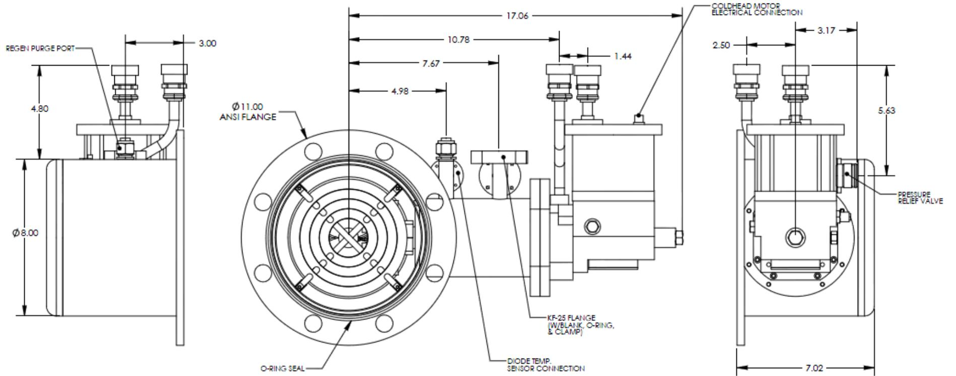
Figure 2 – Cryo-Plex 8LP Cryopump with ANSI Flange Dimension
