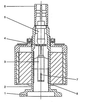
Fig. 3 Sectional view of the PENNINGVAC gauge head PR 25
