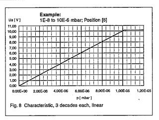
When selecting the "3 decades linear" characteristic, the instrument status can **not** be indicated through the analog signal (3/3; pin 2).
