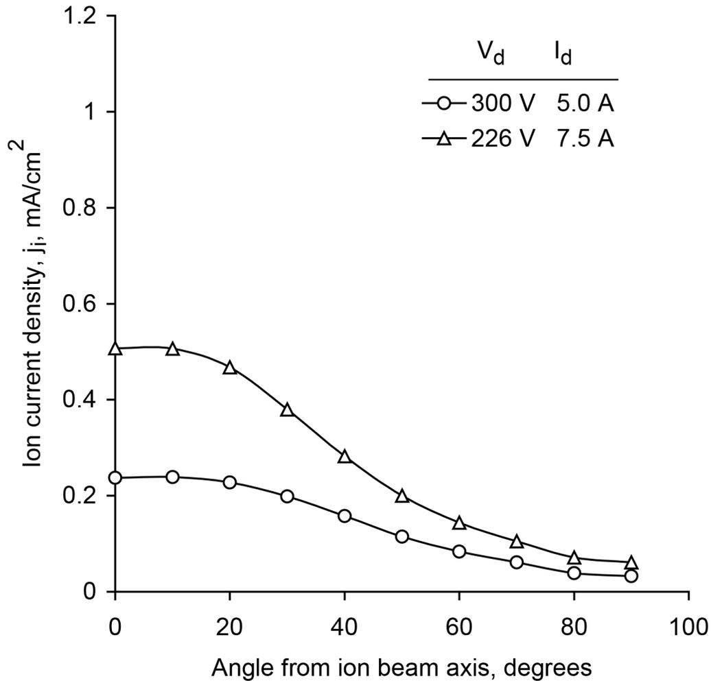
Figure 6-15. Spherical ion current density profiles for the KRI® eH2000HC ion source with the source at the center of the sphere. Source to target distance is 30 cm (12 in.). The working gas is argon.
