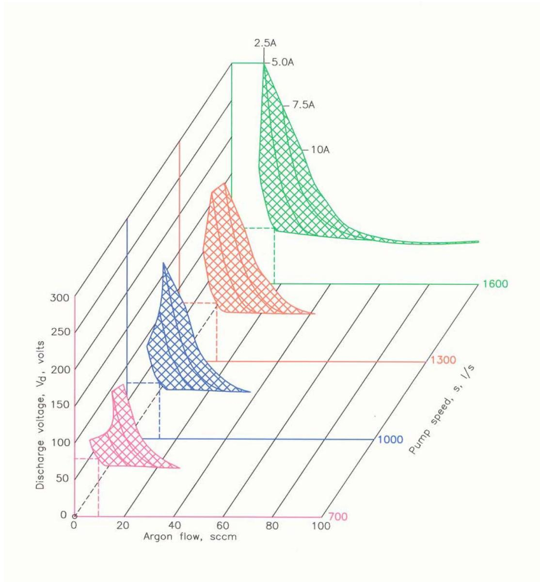
Figure 6-2. Range of operation for the KRI® eH2000HC ion source at various pump speeds, using argon.
