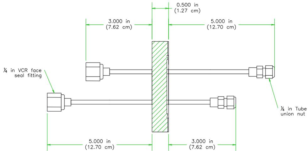
a) 2<sup>3</sup>/<sub>4</sub> inch CF flange gas feedthrough
