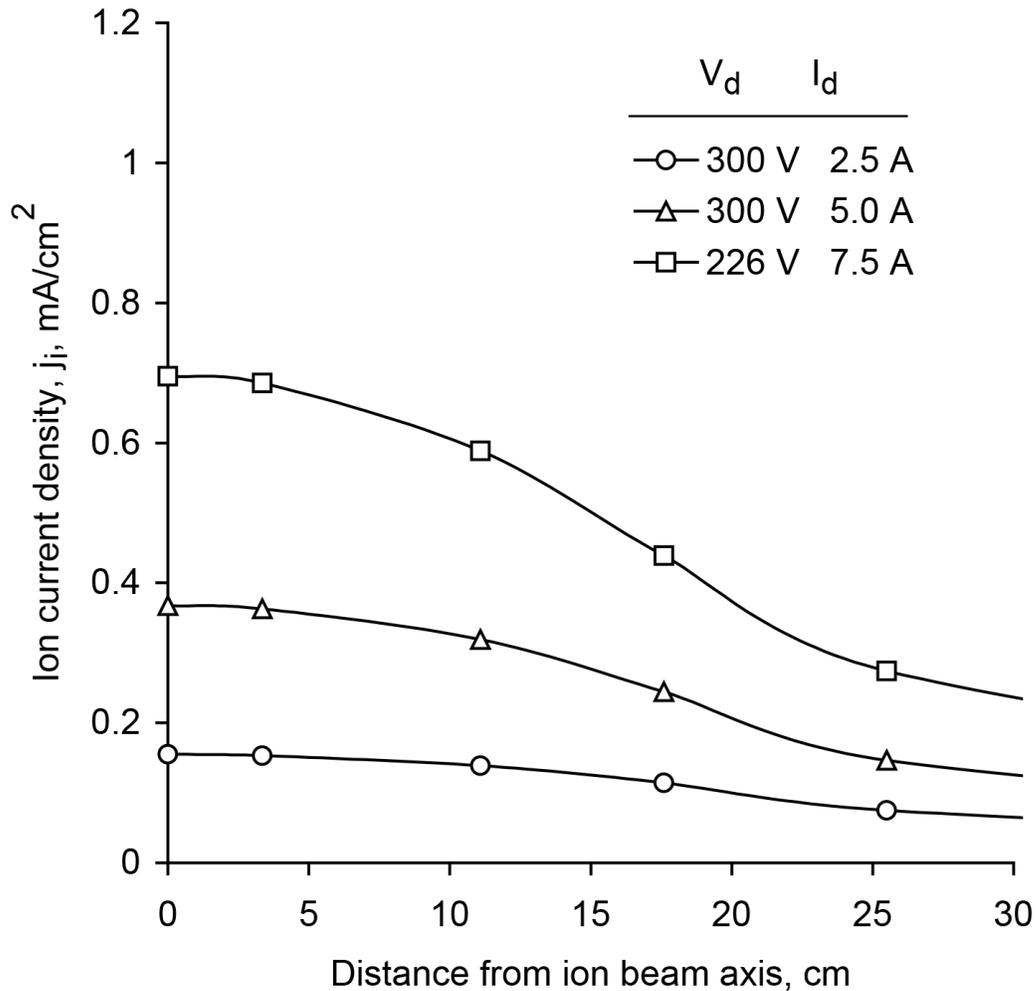
Figure 6-22. Flat target ion current density profiles for the KRI® eH2000HC ion source. Source to target distance is 30 cm (12 in.) and normal to beam axis. The working gas is oxygen.
