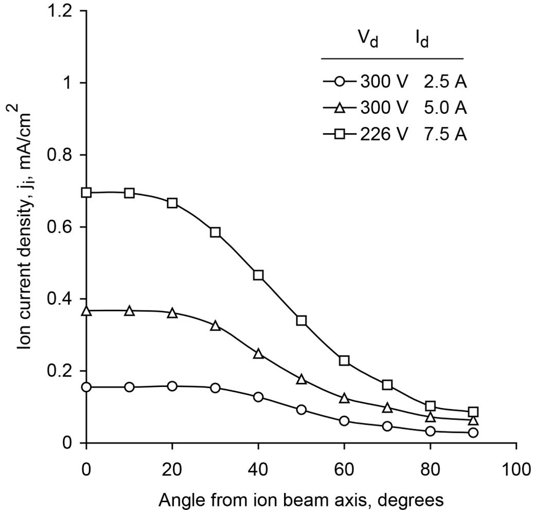
Figure 6-21. Spherical ion current density profiles for the KRI® eH2000HC ion source with the source at the center of the sphere. Source to target distance is 30 cm (12 in.). The working gas is oxygen.
