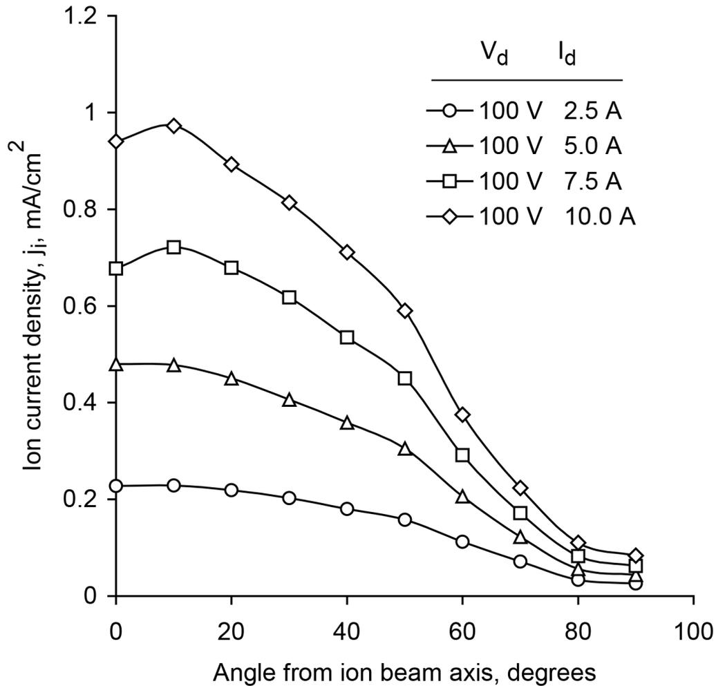
Figure 6-17. Spherical ion current density profiles for the KRI® eH2000HC ion source with the source at the center of the sphere. Source to target distance is 30 cm (12 in.). The working gas is oxygen.
