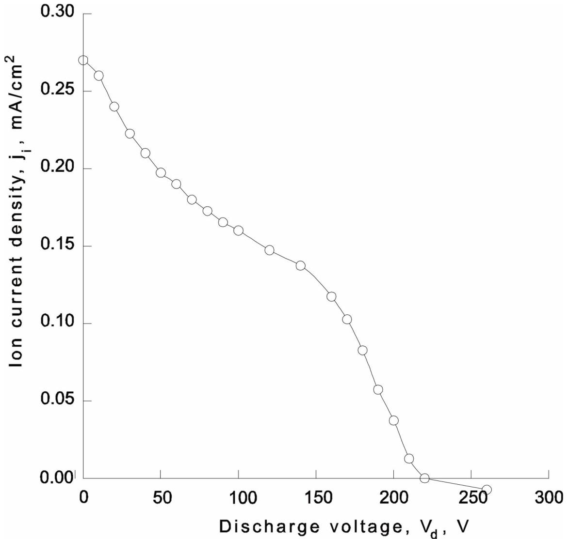
Figure 6-9. Retarding potential probe analysis of the ion beam at a discharge voltage and current of 200 V and 2.8 A.
