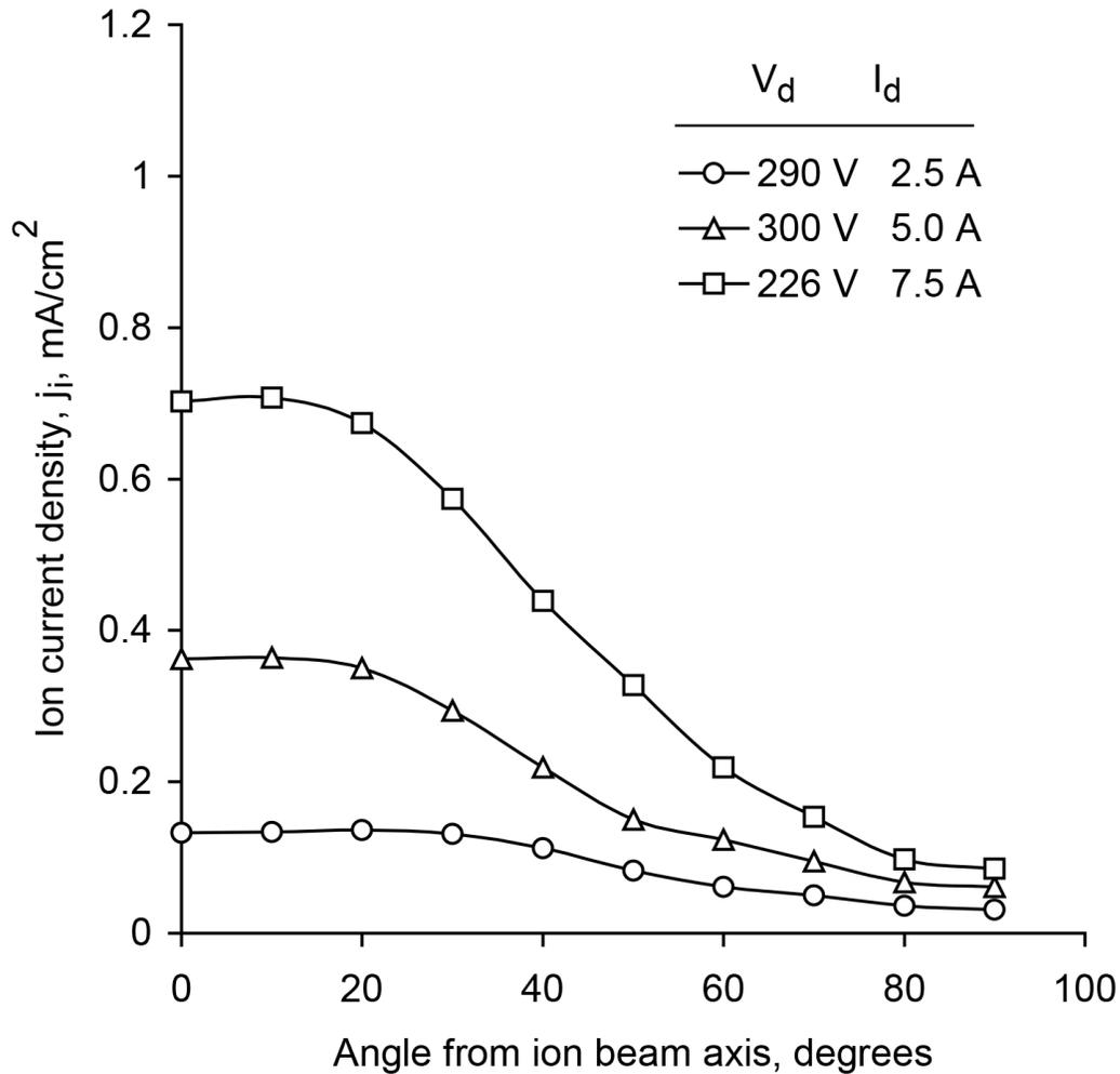
Figure 6-27. Spherical ion current density profiles for the KRI® eH2000HC ion source with the source at the center of the sphere. Source to target distance is 30 cm (12 in.). The working gas is nitrogen.
