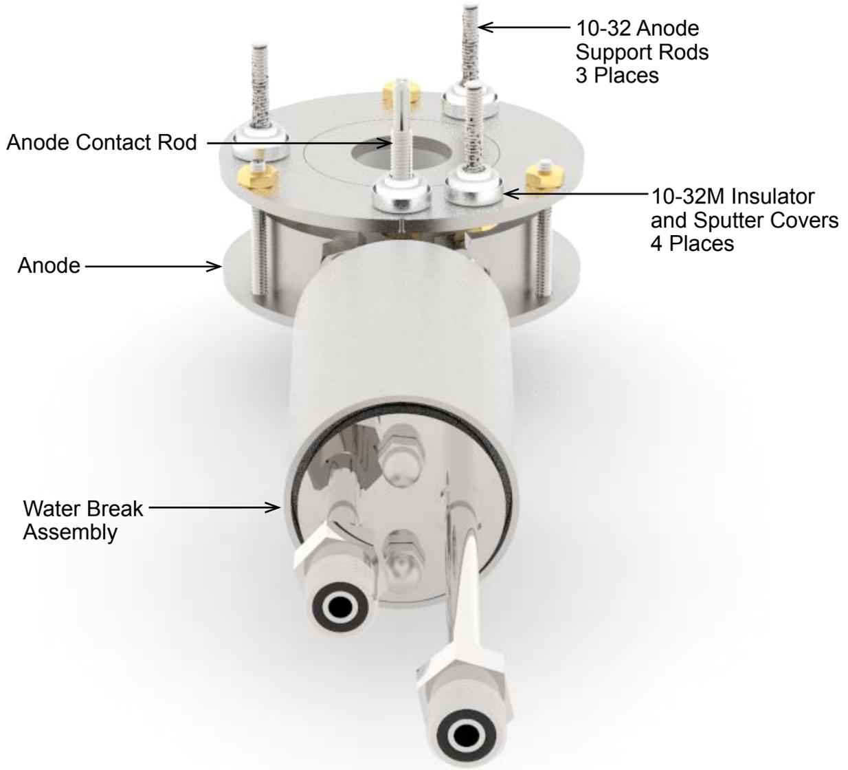
Figure 7-6. Anode support, 10-32M insulators and 10-32 sputter cups.
