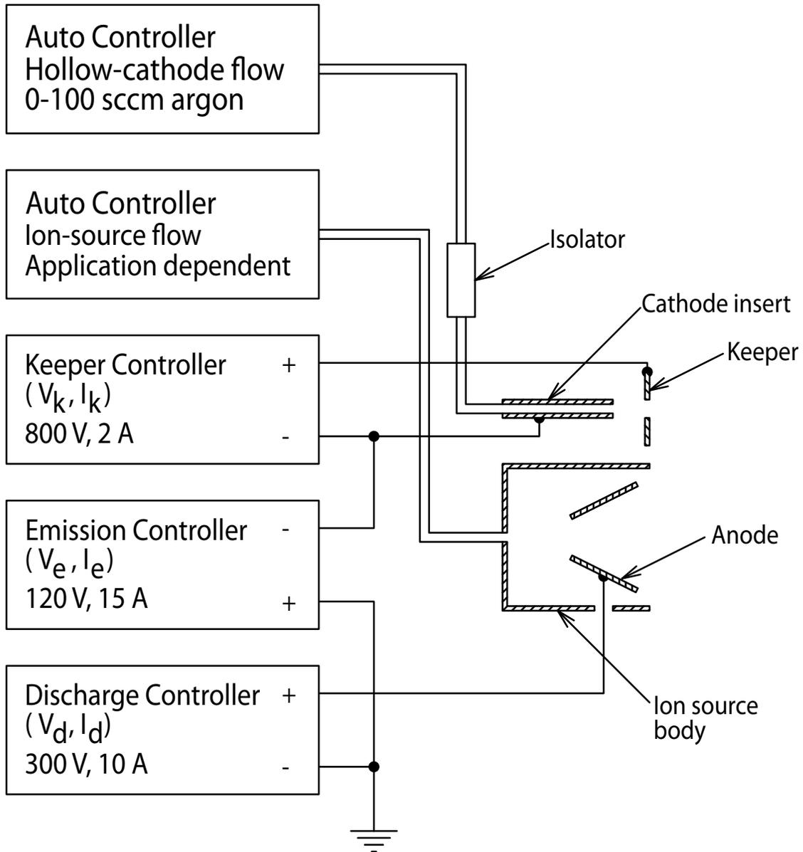
Figure 4-1. Schematic diagram of the eH2000HC ion source and power supplies.
