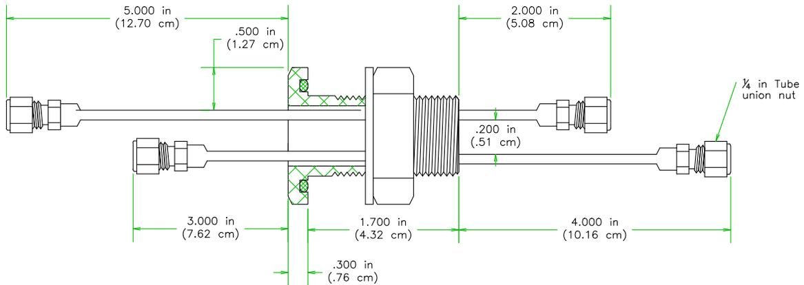
b) 1 inch bolt gas feedthrough
