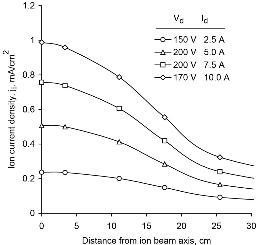
Figure 6-14. Flat target ion current density profiles for the KRI® eH2000HC ion source. Source to target distance is 30 cm (12 in.) and normal to beam axis. The working gas is argon.
