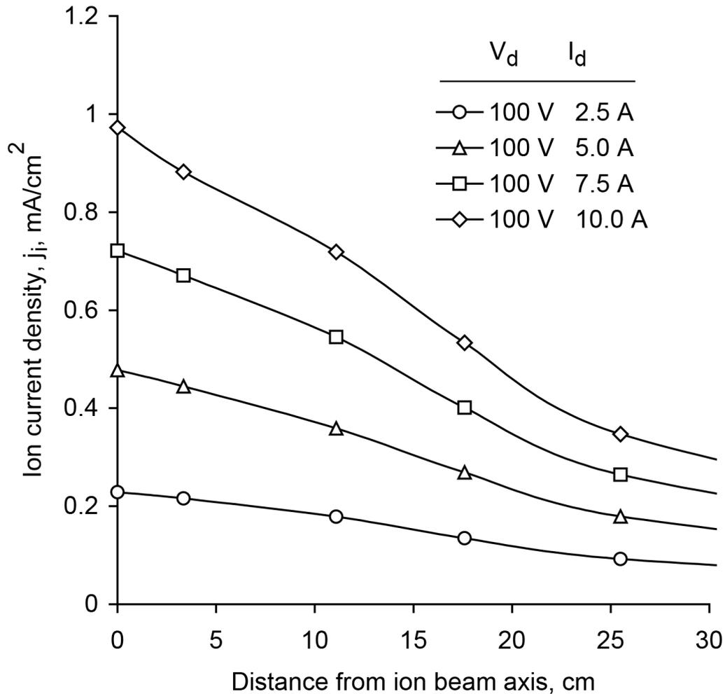
Figure 6-18. Flat target ion current density profiles for the KRI® eH2000HC ion source. Source to target distance is 30 cm (12 in.) and normal to beam axis. The working gas is oxygen.
