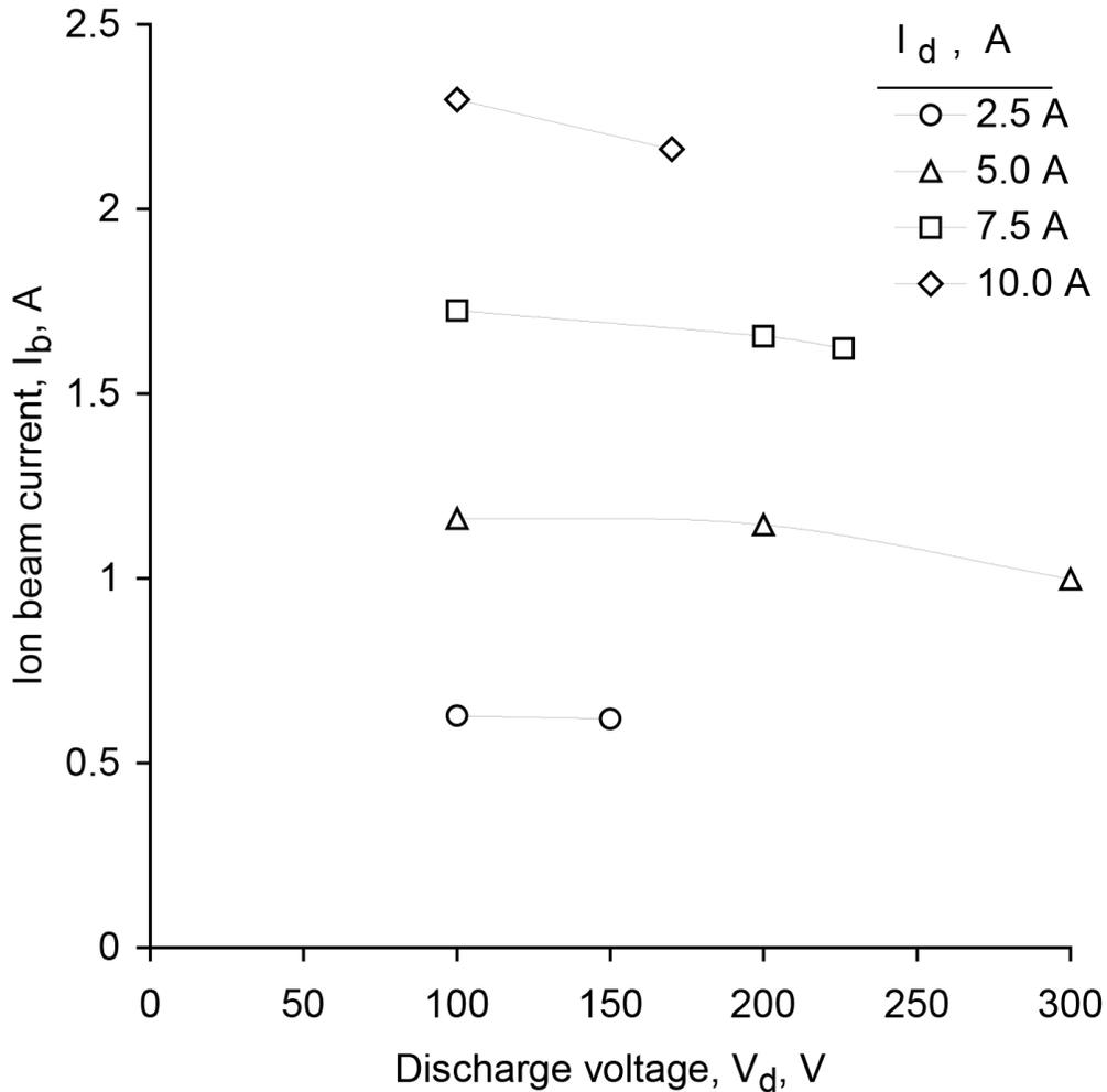
Figure 6-5. Variation of ion beam current with discharge voltage at various discharge currents, using argon.
