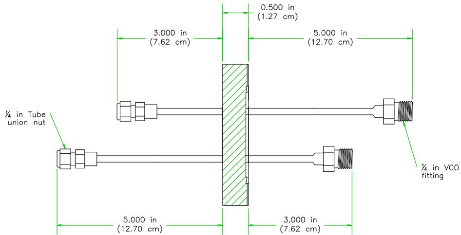
a) 2<sup>3</sup>/<sub>4</sub> inch CF flange water feedthrough
