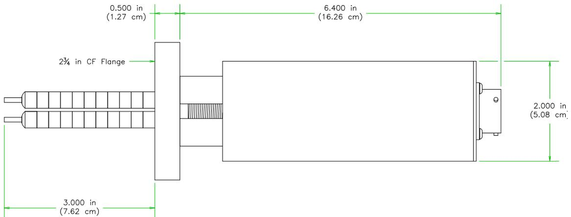
Figure 2-2. 2<sup>3</sup>/<sub>4</sub> CF feedthrough dimensions.
