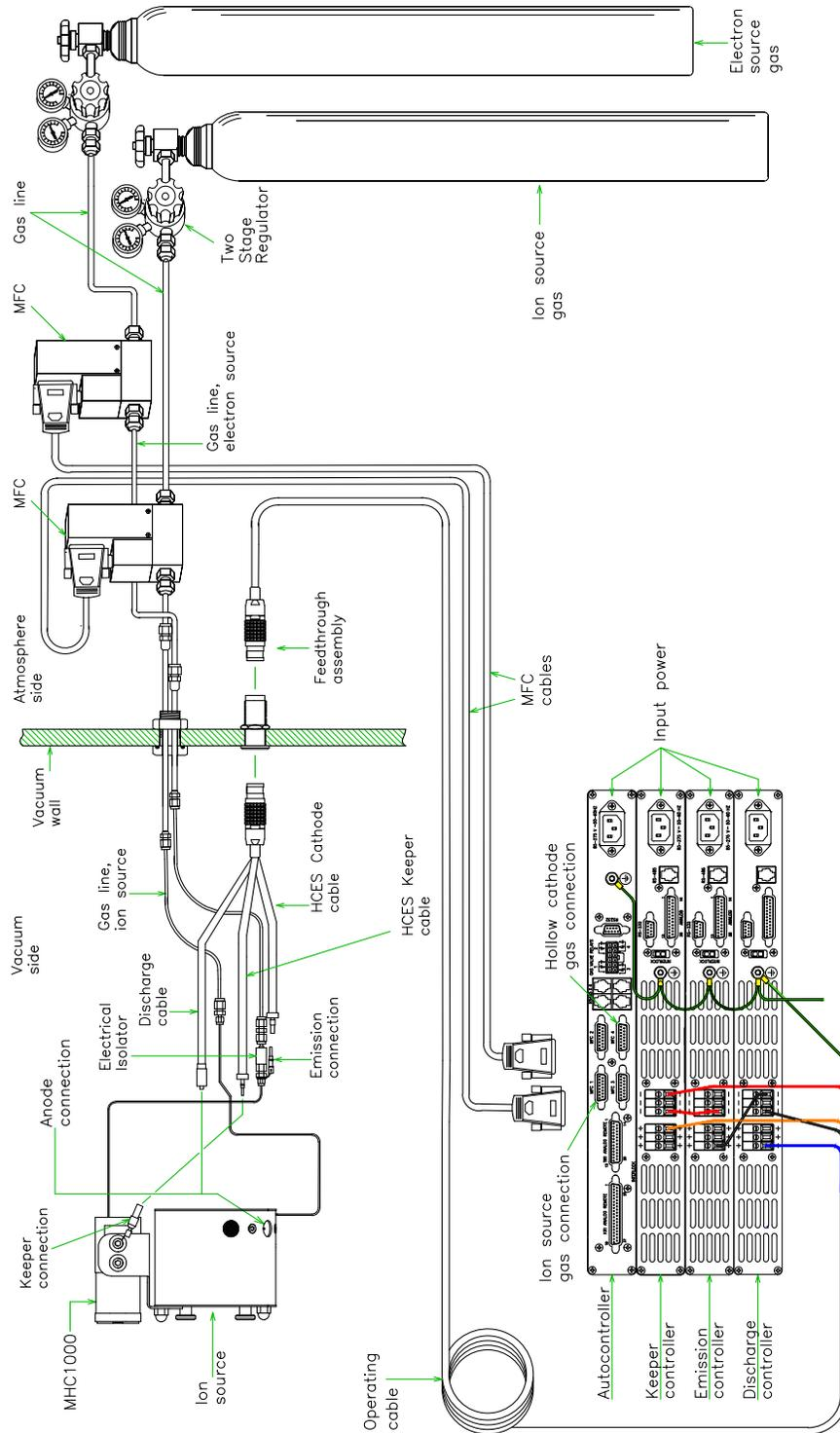
Figure 2-13. Installation drawing for the eH2000HC water-cooled anode with LEMO feedthroughs.
