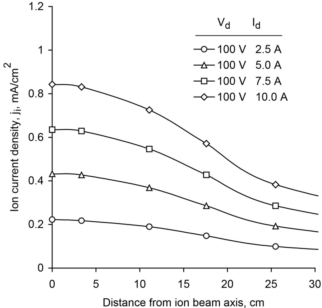
Figure 6-12. Flat target ion current density profiles for the KRI® eH2000HC ion source. Source to target distance is 30 cm (12 in.) and normal to beam axis. The working gas is argon.
