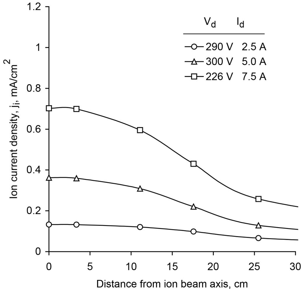
Figure 6-28. Flat target ion current density profiles for the KRI® eH2000HC ion source. Source to target distance is 30 cm (12 in.) and normal to beam axis. The working gas is nitrogen.
