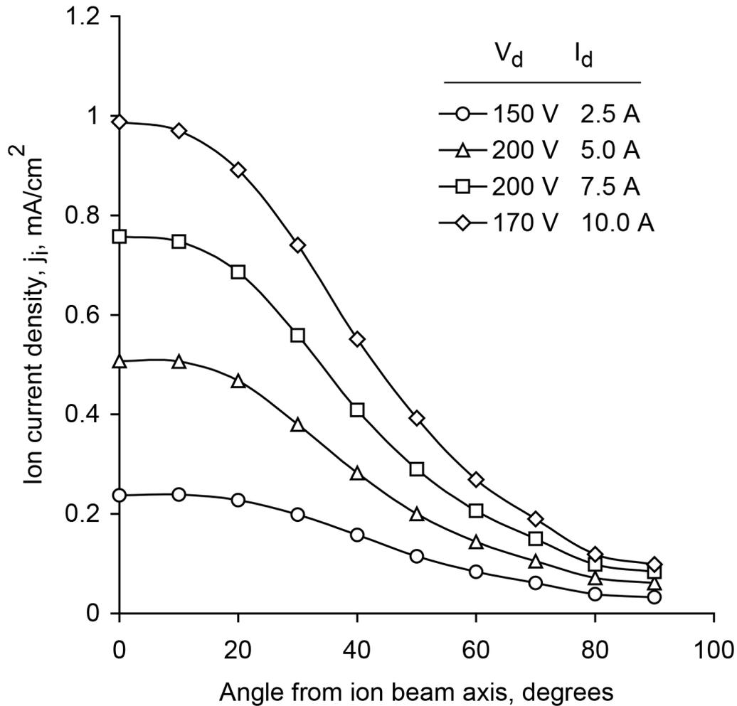
Figure 6-13. Spherical ion current density profiles for the KRI® eH2000HC ion source with the source at the center of the sphere. Source to target distance is 30 cm (12 in.). The working gas is argon.
