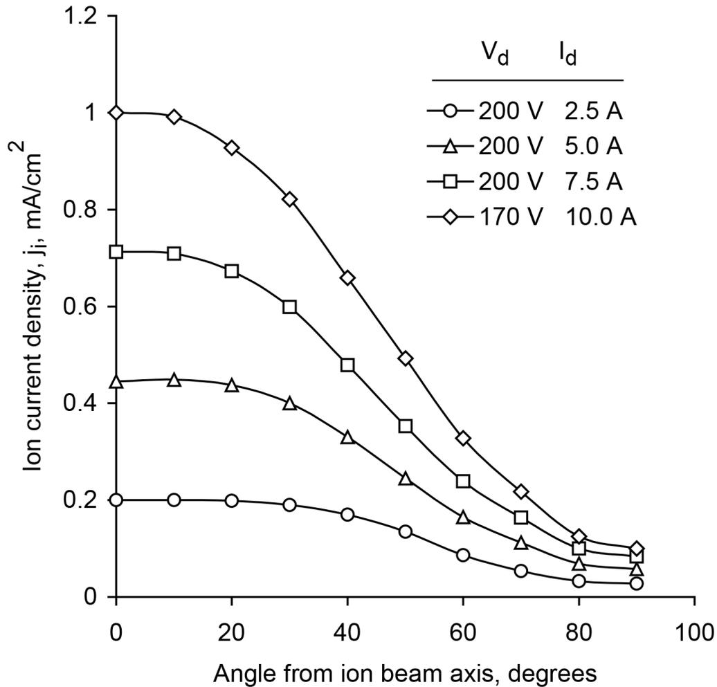
Figure 6-19. Spherical ion current density profiles for the KRI® eH2000HC ion source with the source at the center of the sphere. Source to target distance is 30 cm (12 in.). The working gas is oxygen.
