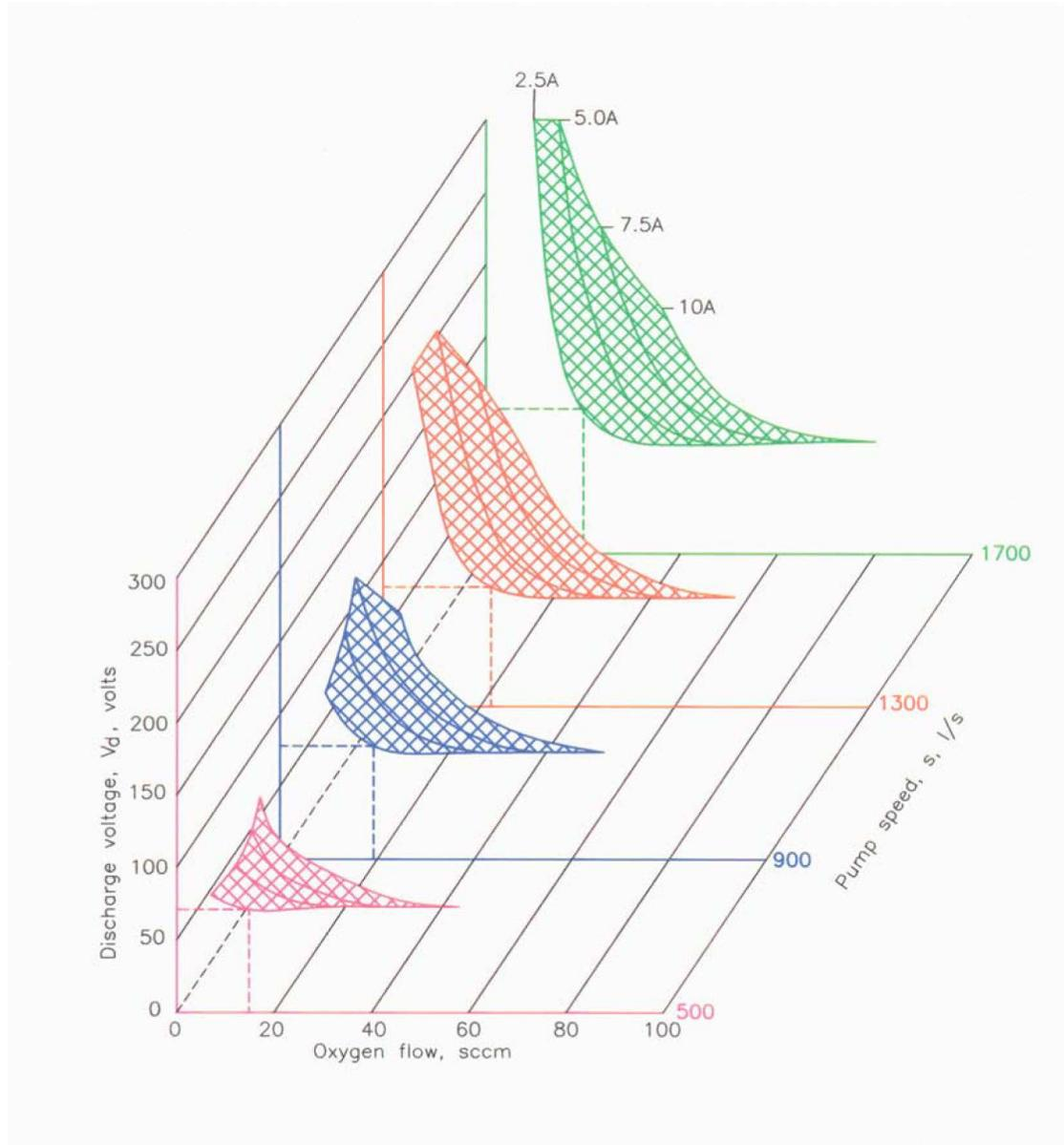
Figure 6-3. Range of operation for the KRI® eH2000HC ion source at various pump speeds, using oxygen.
