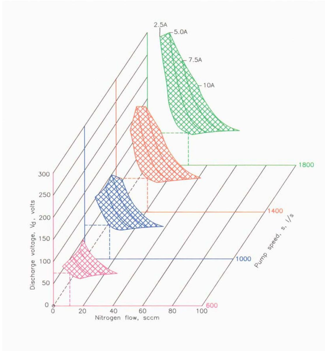
Figure 6-4. Range of operation for the KRI® eH2000HC ion source at various pump speeds, using nitrogen.
