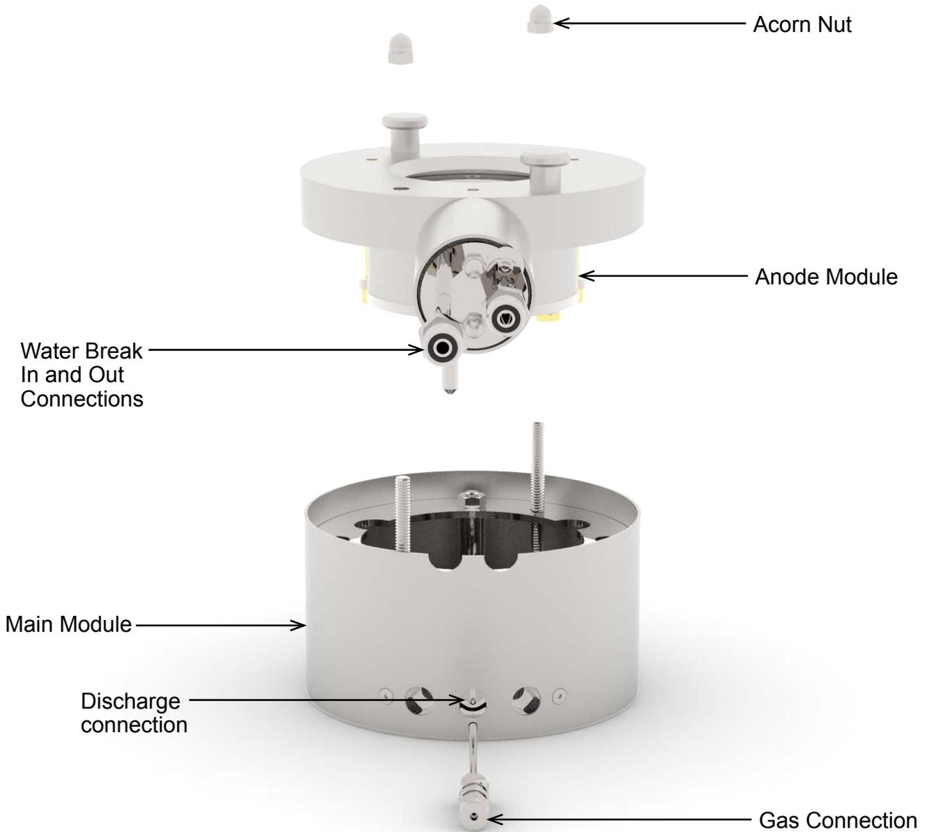
Figure 2-1. The eH2000HC water-cooled anode ion source with the anode module removed.
