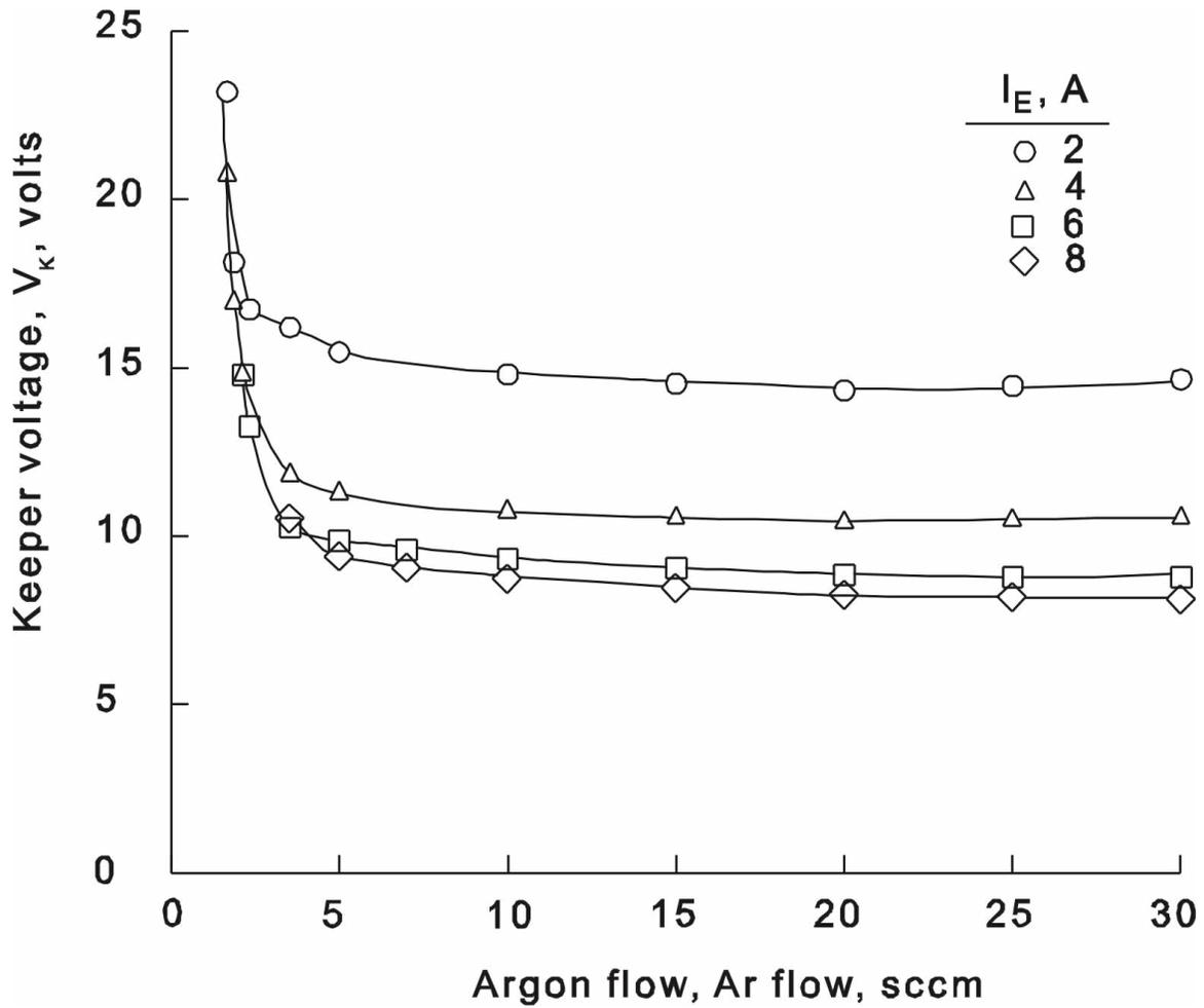
Figure 6-1. Variation in hollow cathode keeper voltage with argon gas flow for various emission currents.
