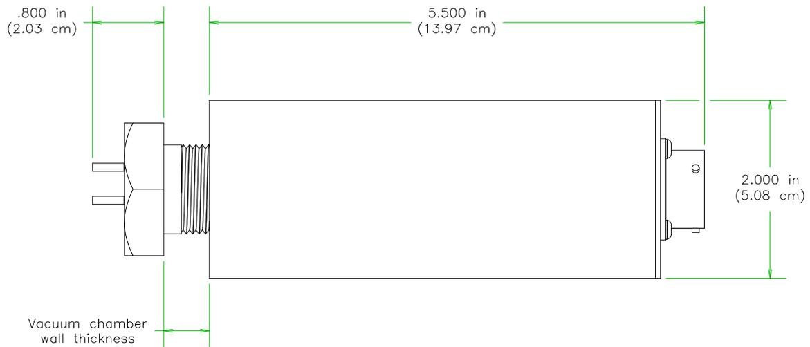
Figure 2-5. 1 inch bolt feedthrough dimensions.
