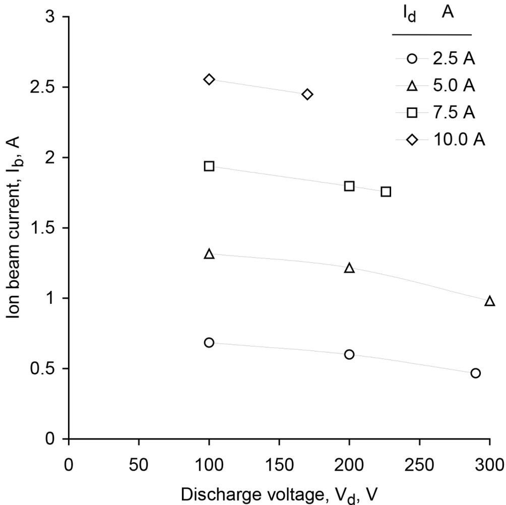
Figure 6-6. Variation of ion beam current with discharge voltage at various discharge currents, using oxygen.
