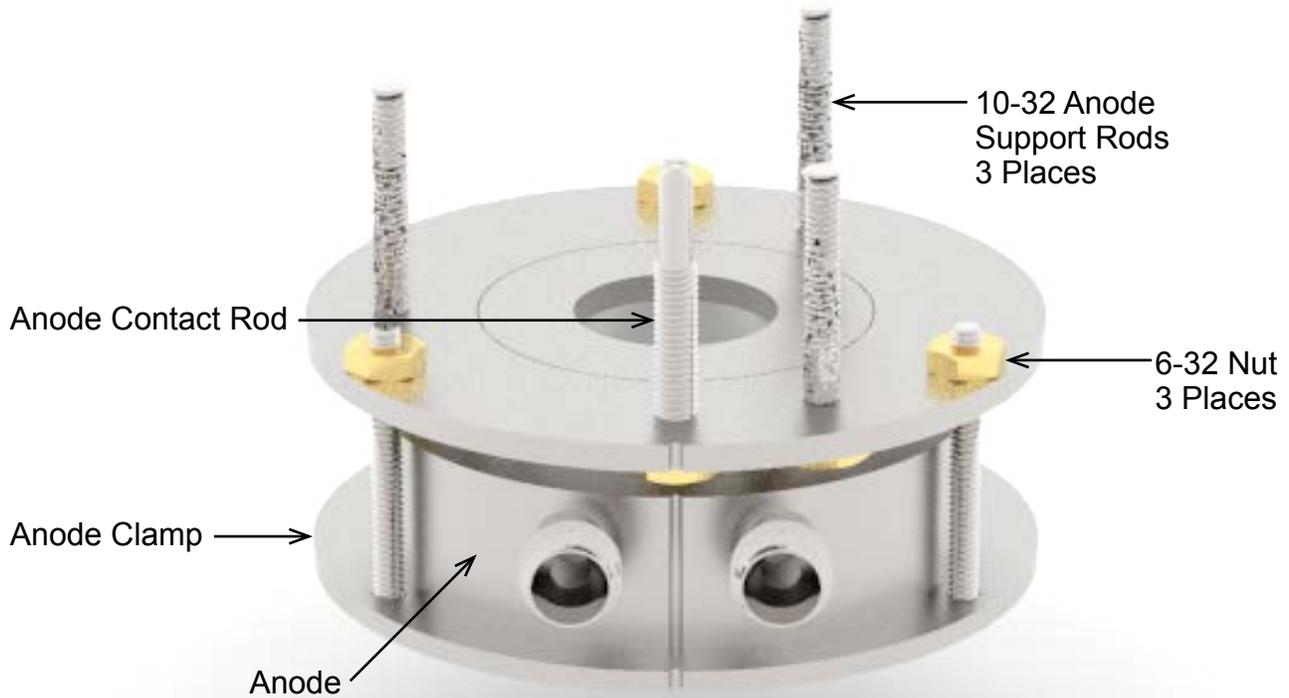
Figure 7-7. Anode and support with water break removed.
