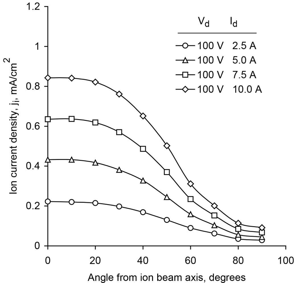
Figure 6-11. Spherical ion current density profiles for the KRI® eH2000HC ion source with the source at the center of the sphere. Source to target distance is 30 cm (12 in.). The working gas is argon.
