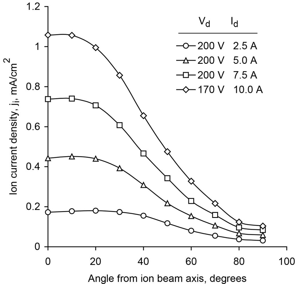
Figure 6-25. Spherical ion current density profiles for the KRI® eH2000HC ion source with the source at the center of the sphere. Source to target distance is 30 cm (12 in.). The working gas is nitrogen.
