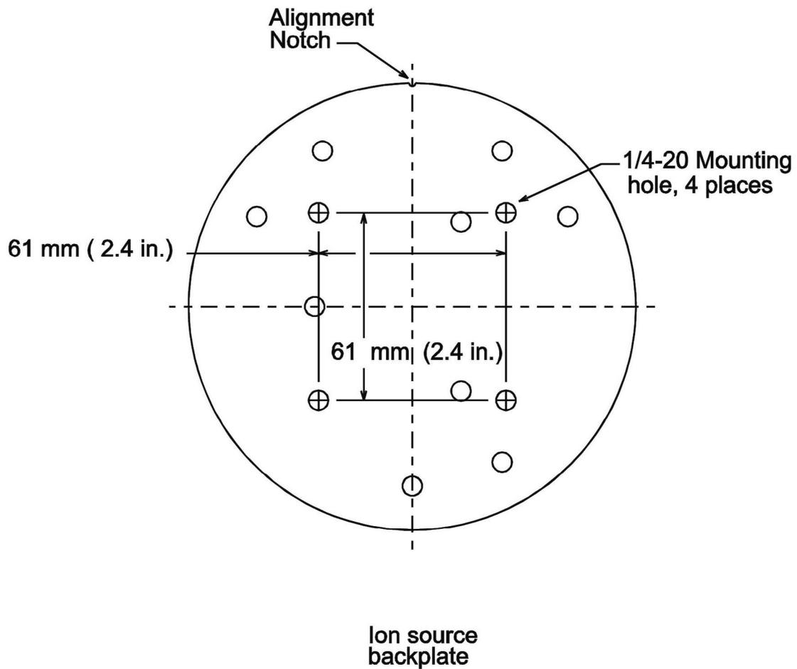
Figure 2-14. Mounting hole locations for the eH2000HC ion source.
