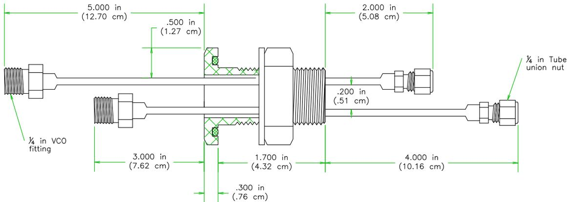
b) 1 inch bolt water feedthrough
