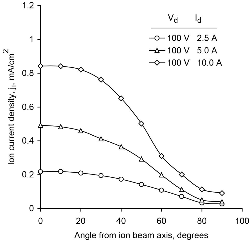
Figure 6-23. Spherical ion current density profiles for the KRI® eH2000HC ion source with the source at the center of the sphere. Source to target distance is 30 cm (12 in.). The working gas is nitrogen.
