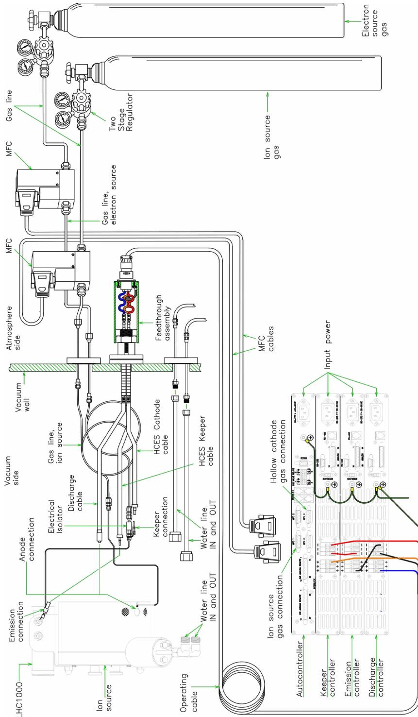
Figure 2-11. Installation drawing for the eH2000HC with CF flange feedthroughs.
