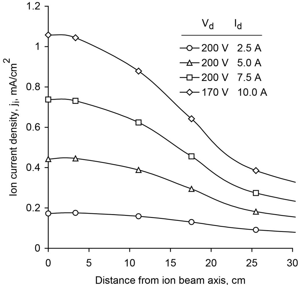
Figure 6-26. Flat target ion current density profiles for the KRI® eH2000HC ion source. Source to target distance is 30 cm (12 in.) and normal to beam axis. The working gas is nitrogen.
