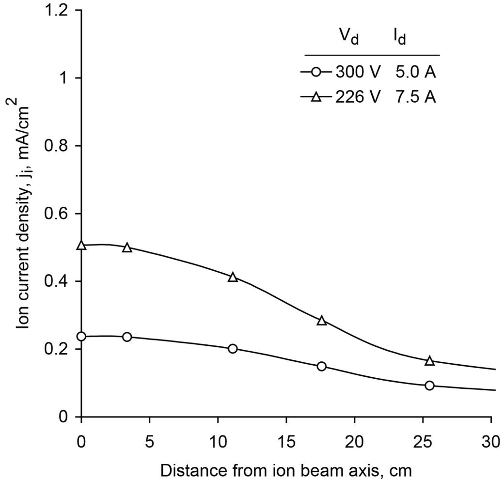
Figure 6-16. Flat target ion current density profiles for the KRI® eH2000HC ion source. Source to target distance is 30 cm (12 in.) and normal to beam axis. The working gas is argon.
