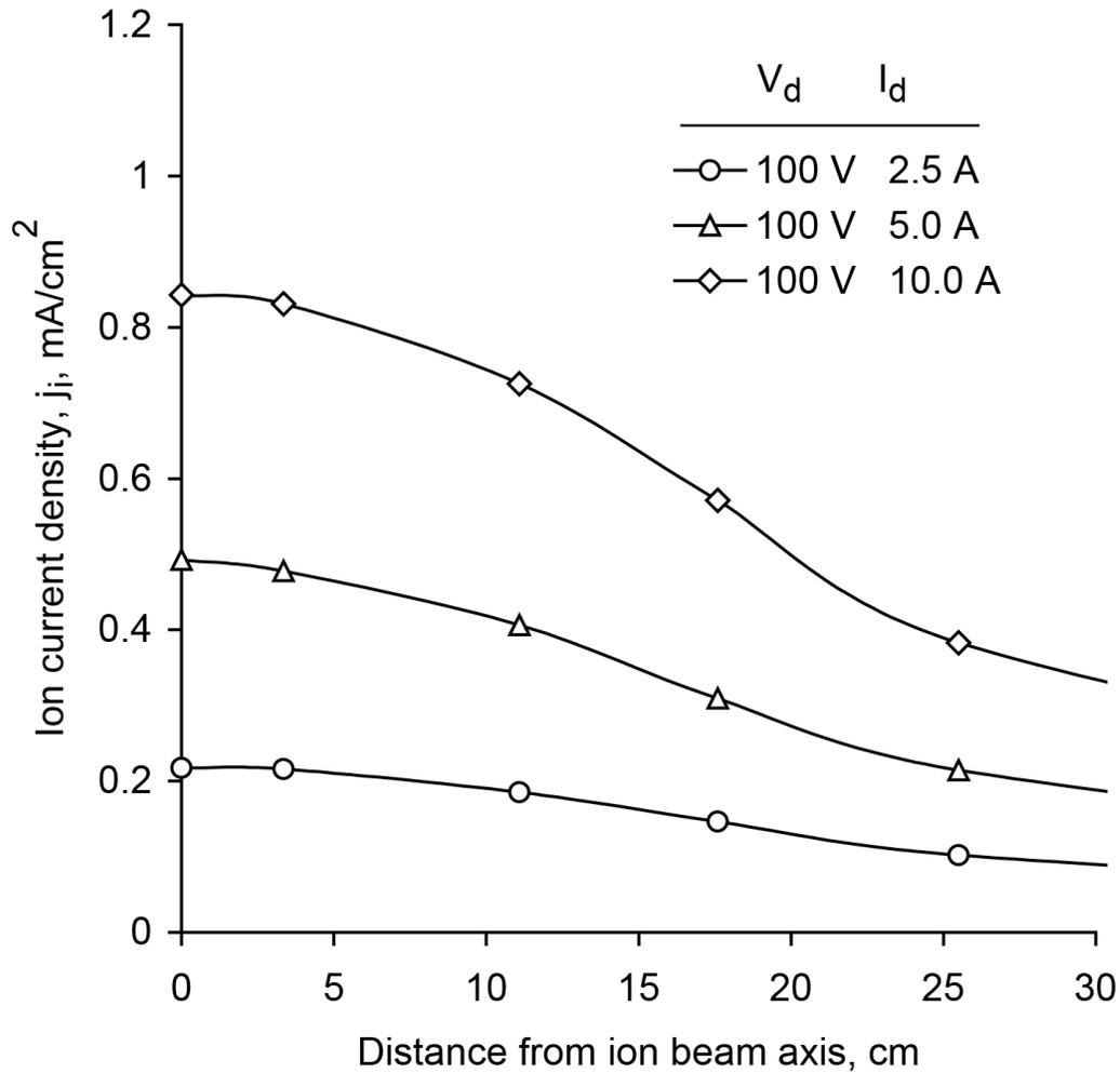
Figure 6-24. Flat target ion current density profiles for the KRI® eH2000HC ion source. Source to target distance is 30 cm (12 in.) and normal to beam axis. The working gas is nitrogen.
