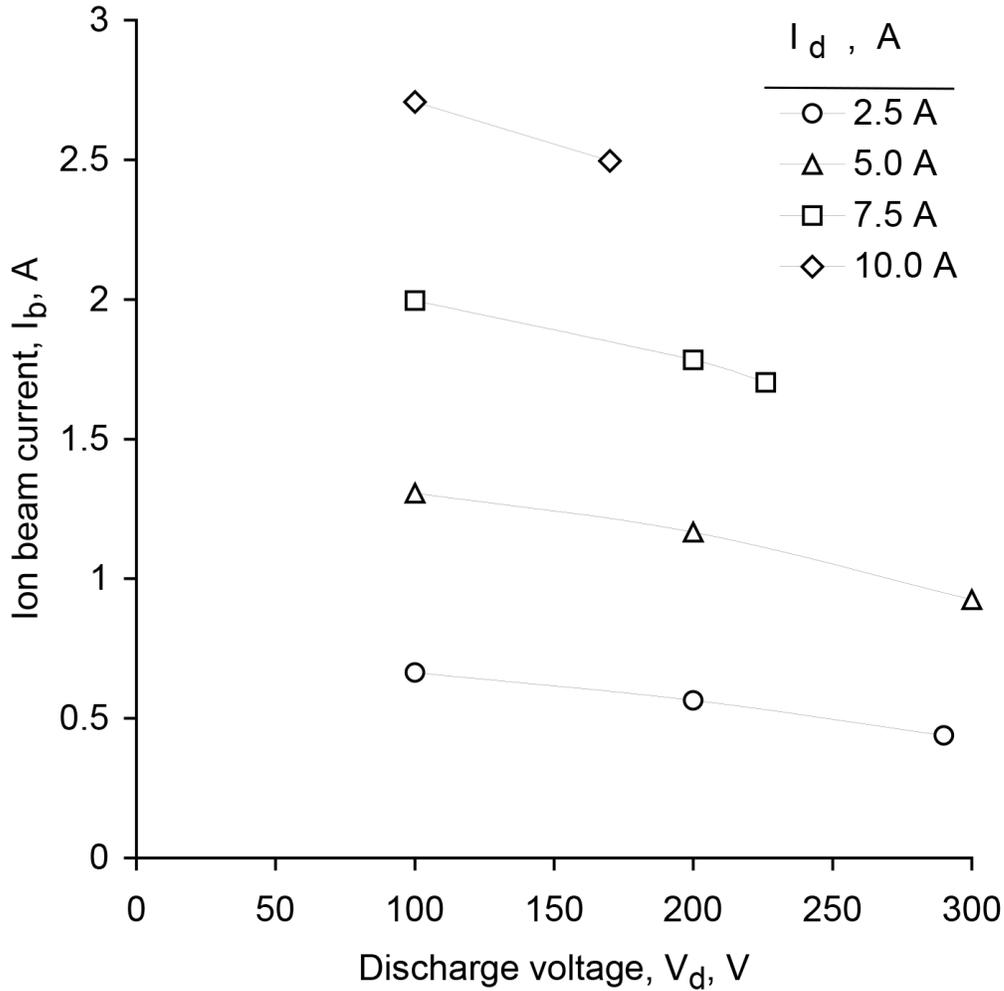
Figure 6-7. Variation of ion beam current with discharge voltage at various discharge currents, using nitrogen.
