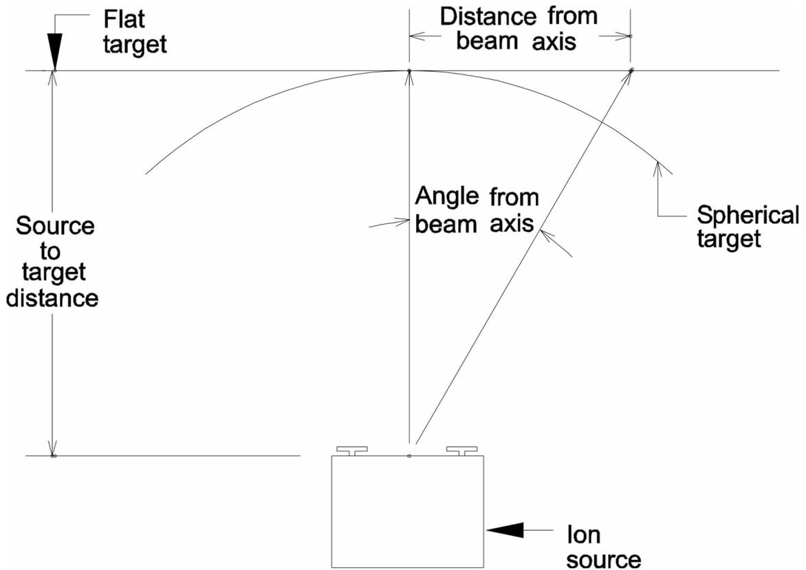
Figure 6-10. Spherical and flat target configurations.
