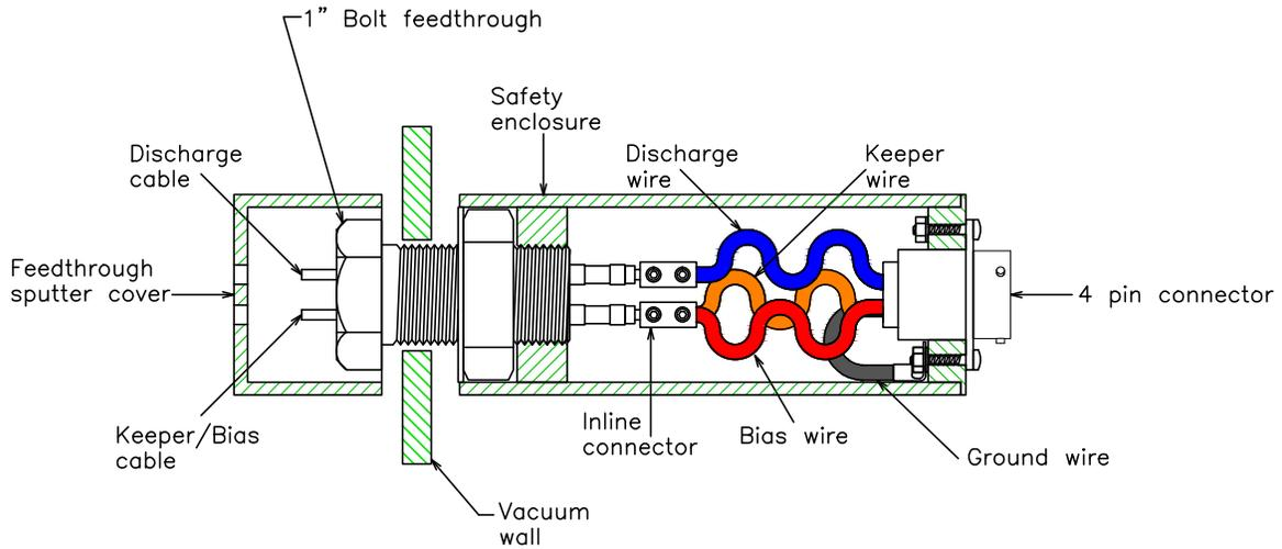
a) Cutaway view of the electrical feedthrough assembly.
