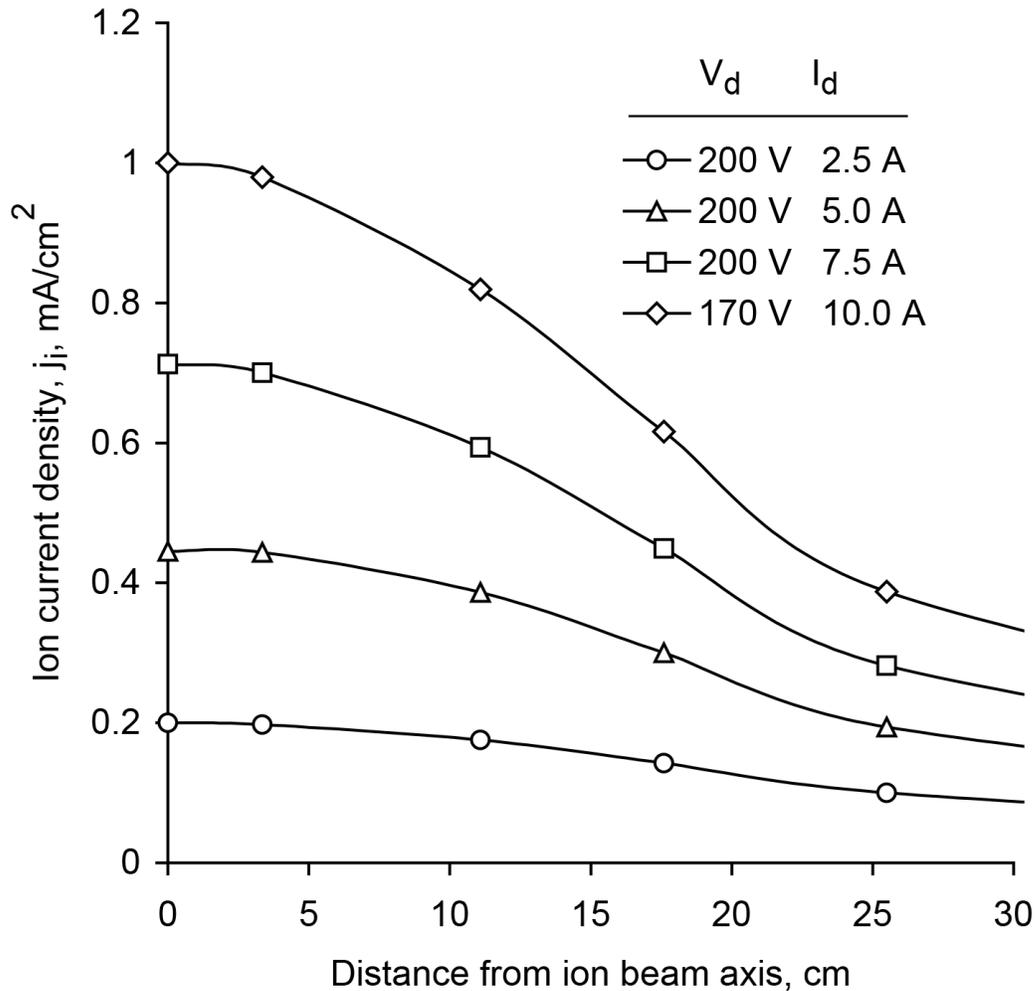
Figure 6-20. Flat target ion current density profiles for the KRI® eH2000HC ion source. Source to target distance is 30 cm (12 in.) and normal to beam axis. The working gas is oxygen.
