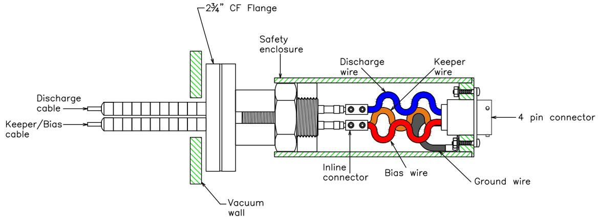
a) Cutaway view of the electrical feedthrough assembly.
