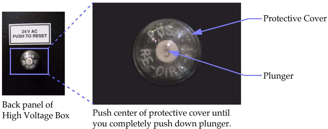
Figure 7-8: *Control voltage circuit breaker*
