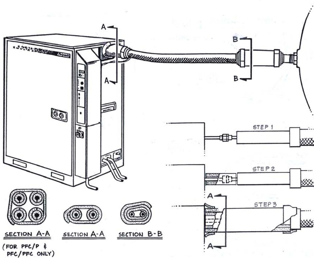
Figure 3-25: Insulating Exposed Tubes and Couplings Method
