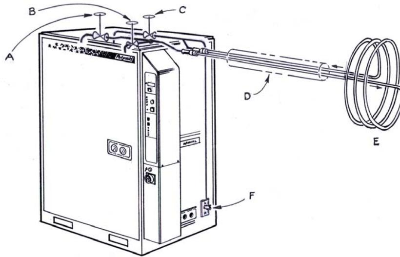
Figure 3-17: Evacuation Valve, Refrigerant Line & Cryosurface Relationship
