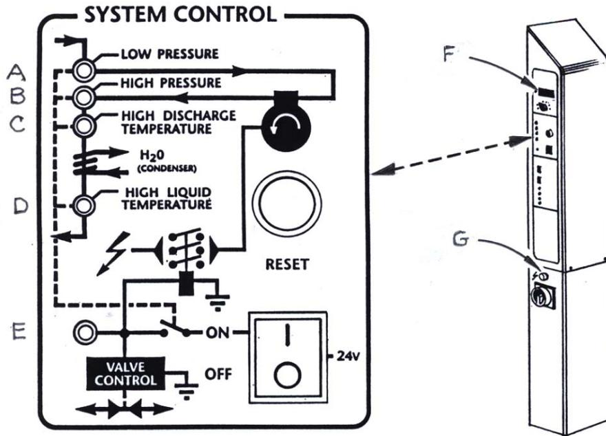
Figure 7-1: Unit indicator lamps
