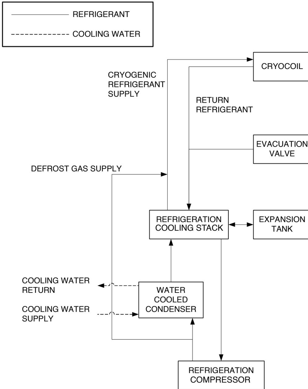
Figure 3-7: System Block Diagram
