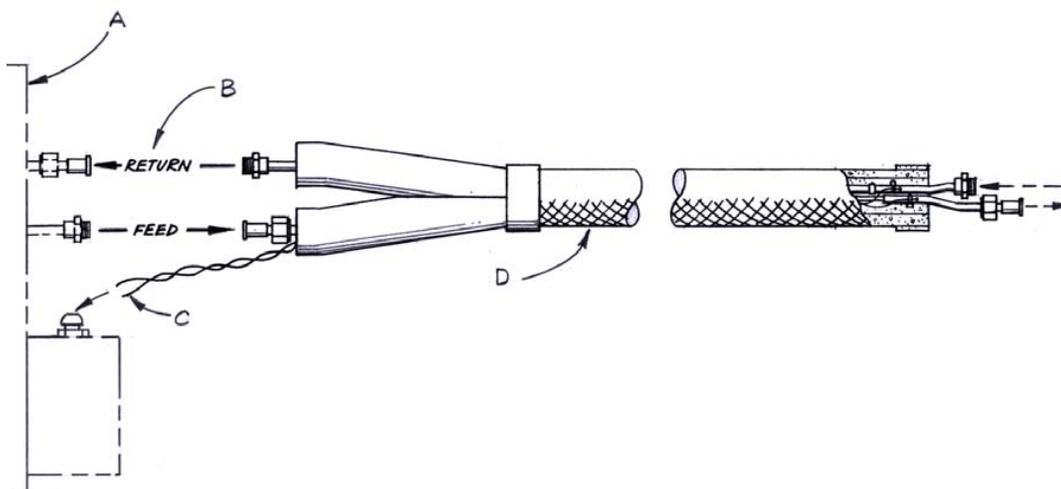
Figure 3-15: Refrigerant line connection
