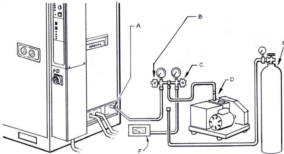
*Figure 3-20: Refrigerant Line & Cryosurface—Evacuation Set-up*
