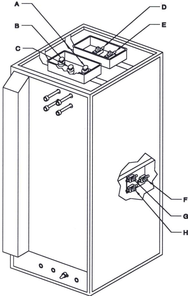
Figure 1-5: Location of isolation & solenoid valves
