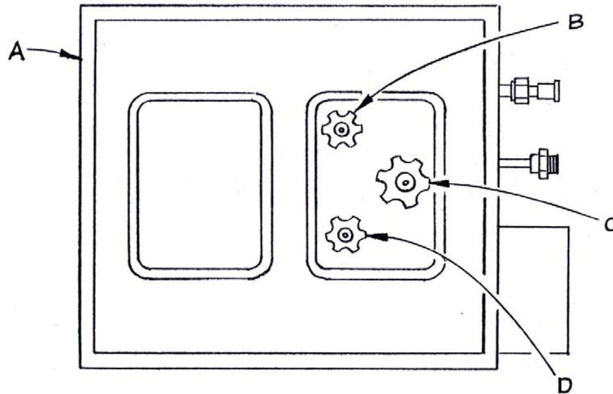
Figure 3-16: Isolation Valves Location
