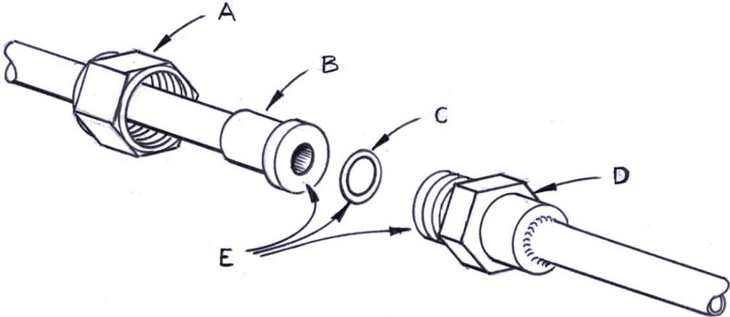
Figure 3-13: Parker CPI UltraSeal coupling (standard fitting)
