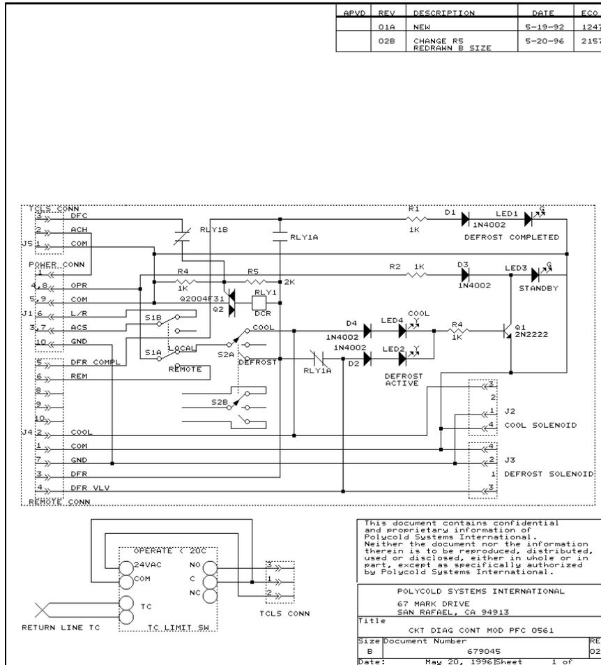
Figure 10-5: PFC Refrigerant Circuit Controls
