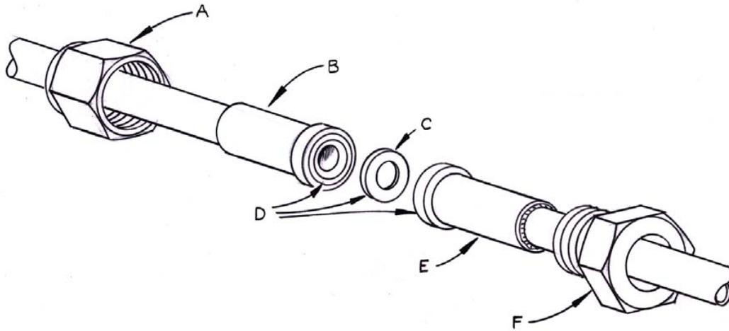
Figure 3-14: Cajon VCR Coupling (optional fitting)
