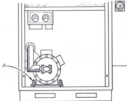
Figure 3-8: Location of Compressor Hold-down Nuts
