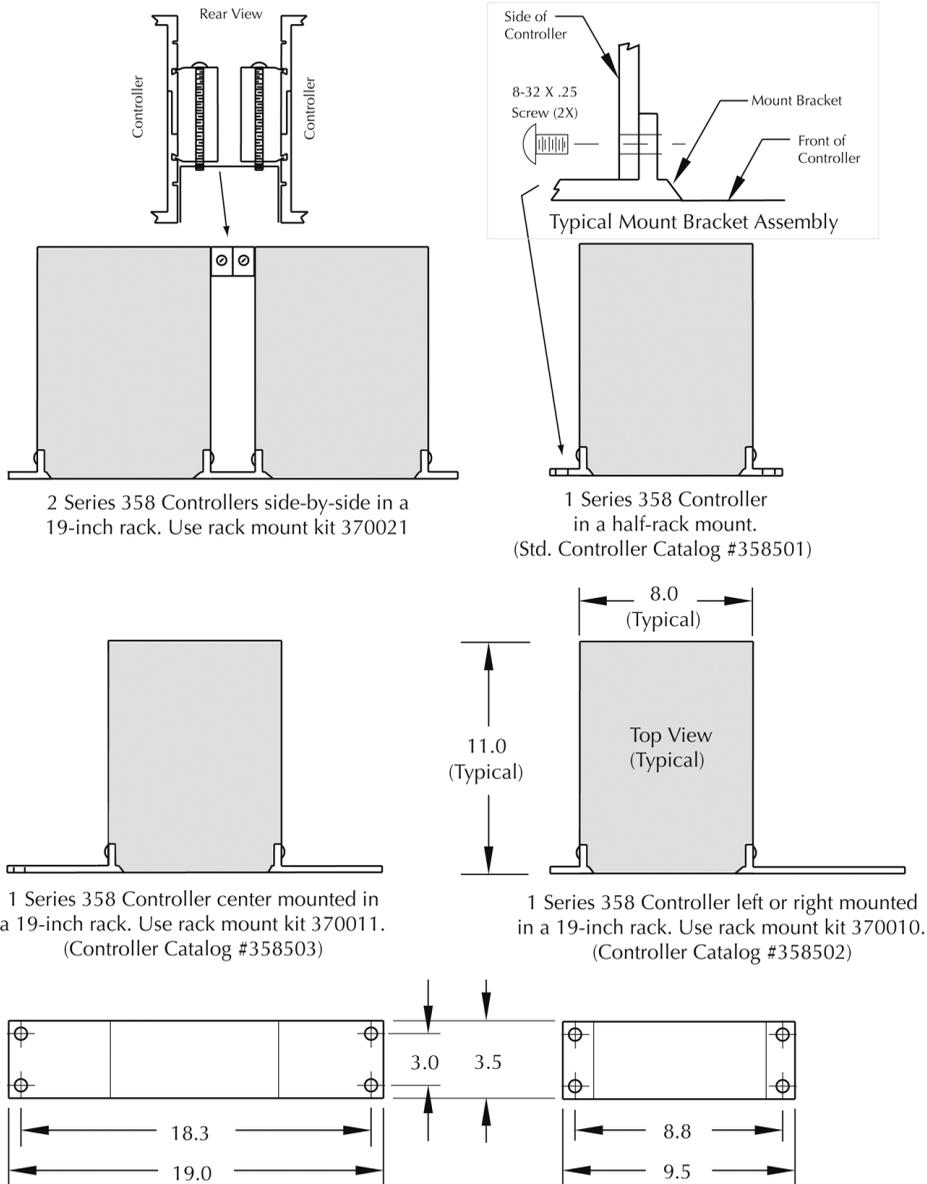
2 Series 358 Controllers side-by-side in a 19-inch rack. Use rack mount kit 370021
