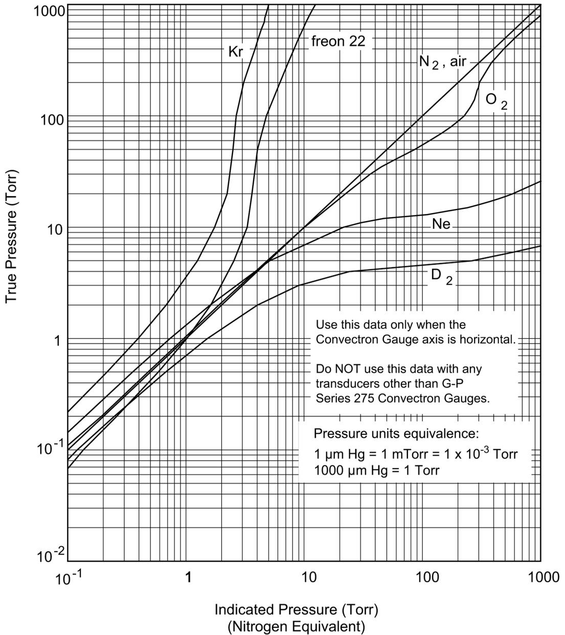
Figure 5-9 True Pressure versus Indicated Pressure for Commonly used Gases,  $10^{-4}$  to  $10^{-1}$  mbar
