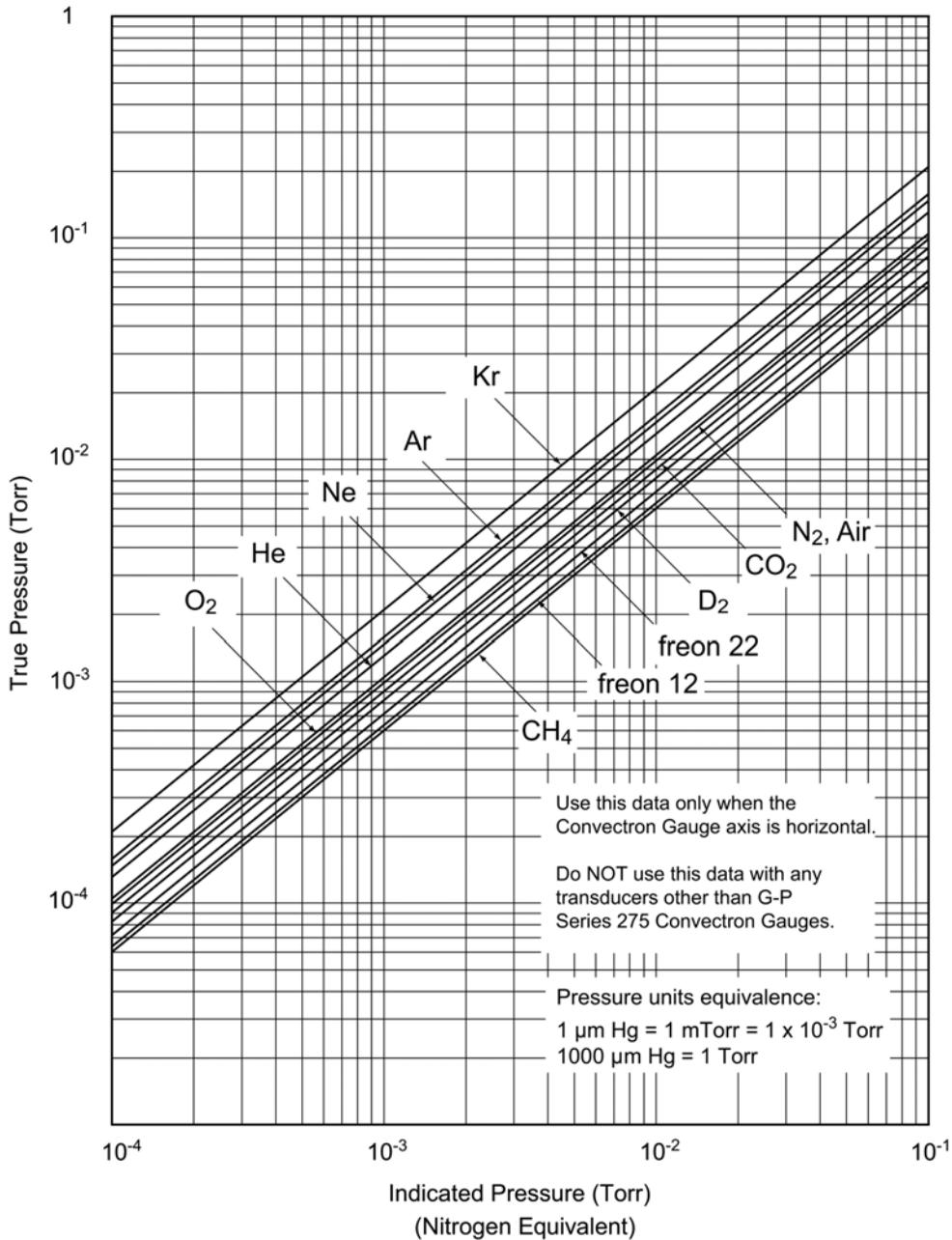
Figure 5-7 True Pressure versus Indicated Pressure for Commonly used Gases,  $10^{-1}$  to 1000 Torr
