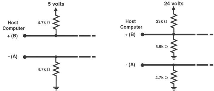
Figure 3-14 RS-485 Wiring Connector
