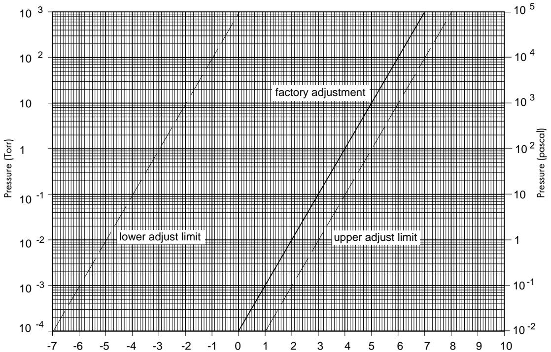
The voltage signal is smooth and continuous throughout all the decades of pressure measurement. This format is useful for computerized data acquisition because a simple equation (finding the common antilogarithm) may be programmed to calculate pressure from the voltage output.
