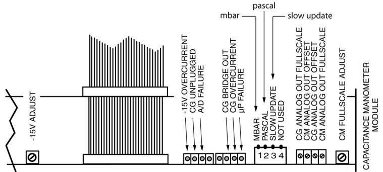
**Figure 4-6 Capacitance Manometer Wiring Diagram**
