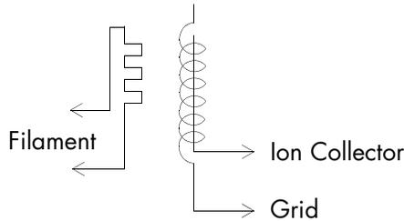
When an energetic electron collides with a gas molecule an electron may be dislodged from the molecule leaving it with a positive charge. Most ions are then accelerated to the collector. The rate at which electron collisions with molecules occur is proportional to the density of gas molecules, and hence the ion current is proportional to the gas density (or pressure, at constant temperature).
