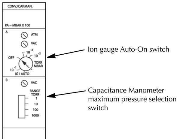
Use the IG AUTO potentiometer to set the auto turn ON pressure for the Micro-Ion Gauge. The IG AUTO turn-on potentiometer is marked with rough pressure calibration markings. To set the pressure at which the Micro-Ion Gauge will turn ON with falling Convectron pressure, and OFF with rising Convectron pressure, simply adjust the potentiometer to point to the desired pressure.
