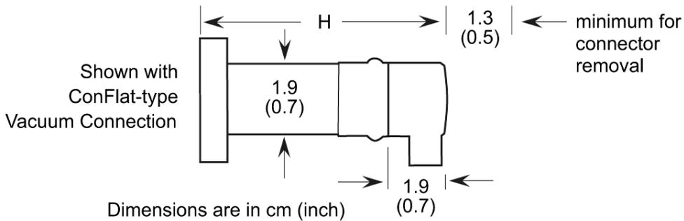
The dimensions of the Convectron gauge are shown Figure 2-10. Dimensions are in cm (in.). J dimensions are given in Table 2-4.
