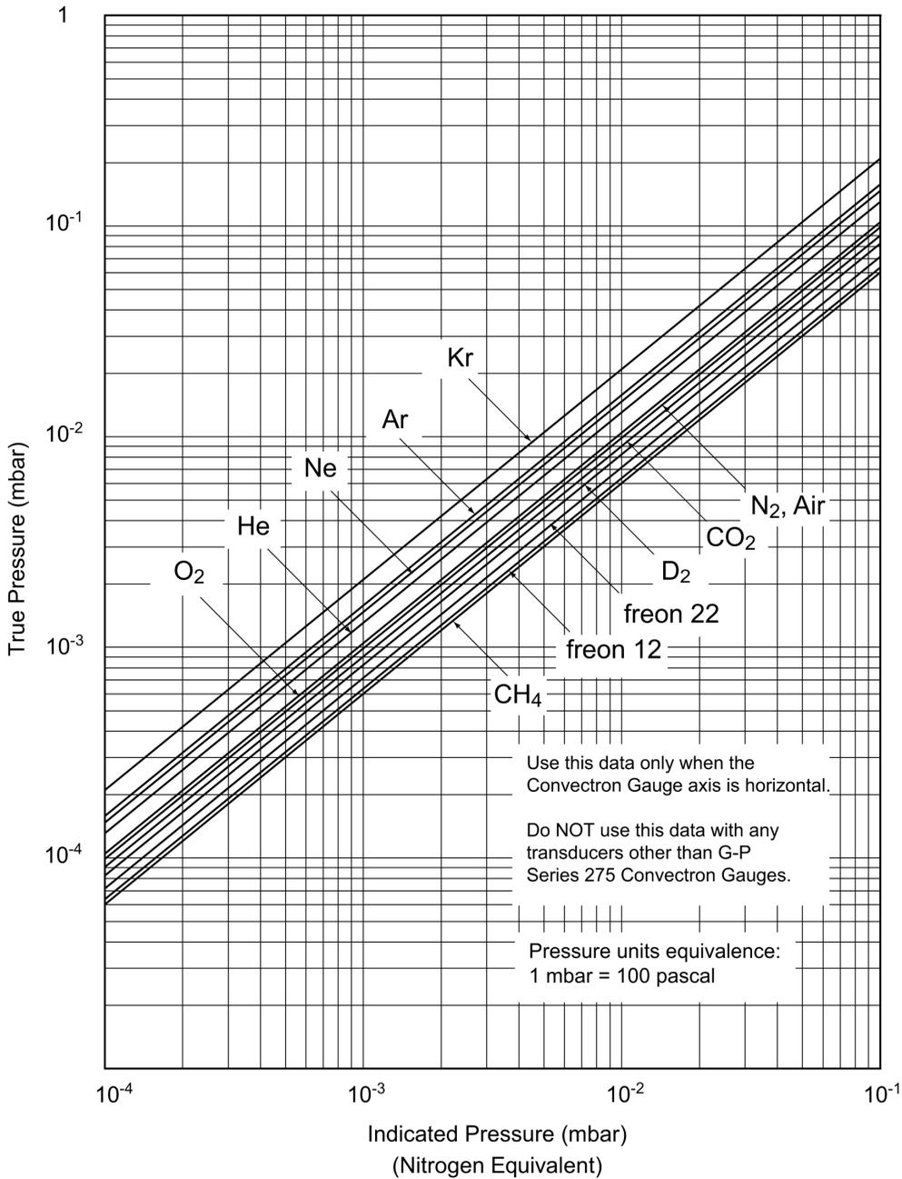
Figure 5-10 True Pressure versus Indicated Pressure for Commonly used Gases,  $10^{-1}$  to 1000 mbar
