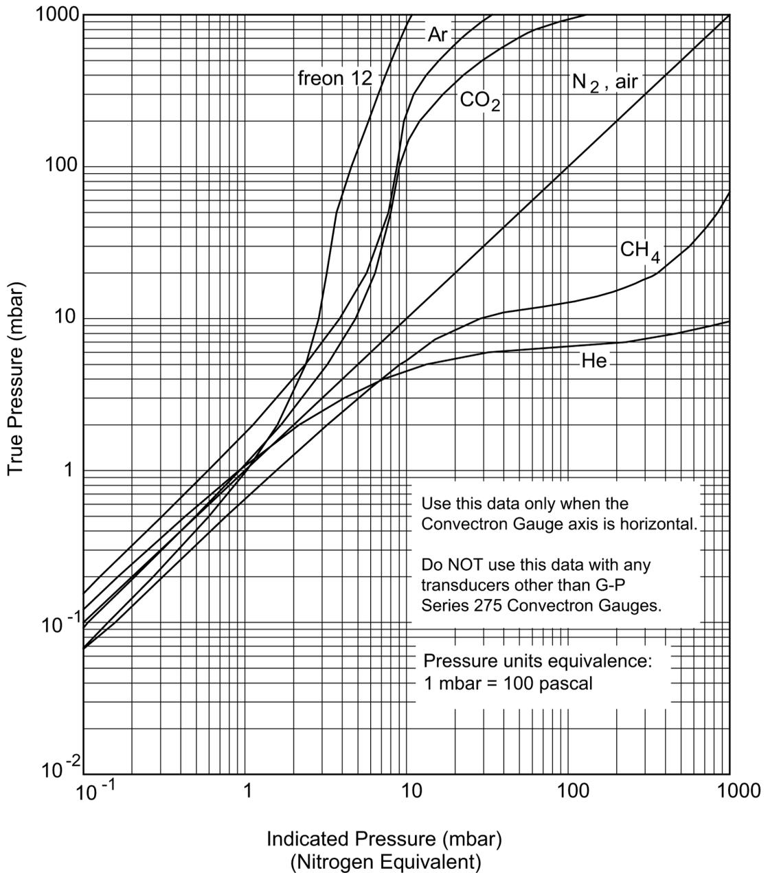
Figure 5-11 True Pressure versus Indicated Pressure for Commonly used Gases, 10<sup>-1</sup> to 1000 mbar
