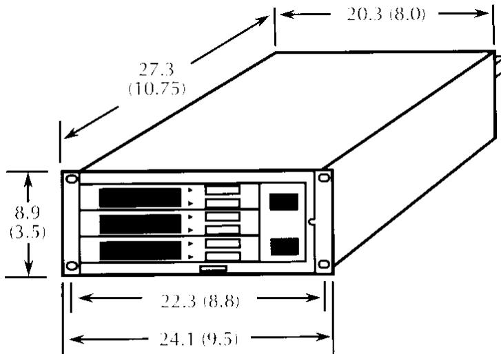
The dimensions of the Micro-Ion gauge are shown in Figure 2-9. Dimensions are in cm (in.). H dimensions are given in Table 2-4.
