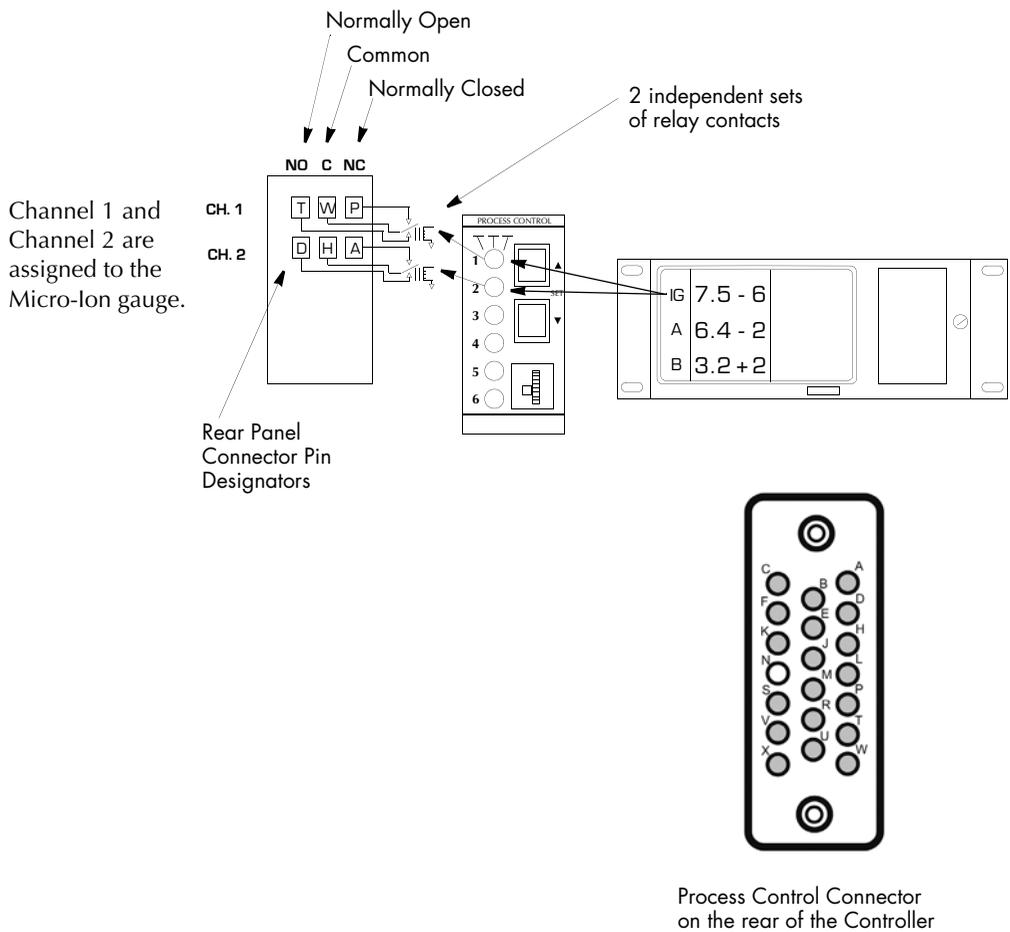
Figure 3-9 6-Channel Process Control Option Card
