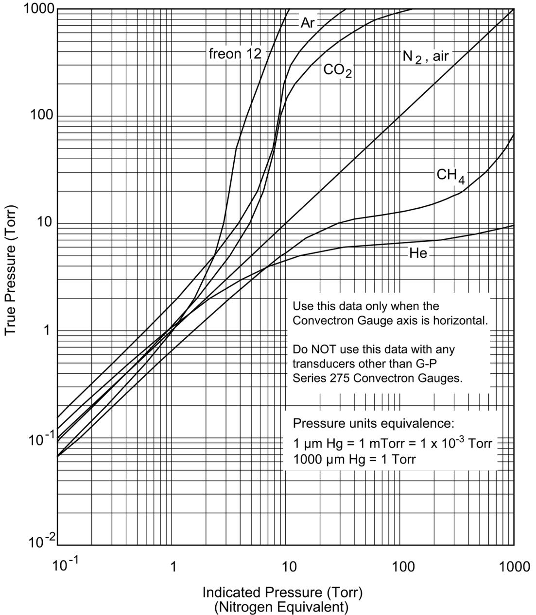
Figure 5-8 True Pressure versus Indicated Pressure for Commonly used Gases,  $10^{-1}$  to 1000 Torr
