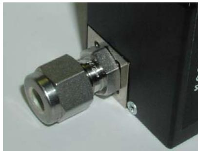
Prior to installation, make certain all tubing is clean and free of obstructions. Install the tubing in such a manner that permits removal if the MFC when necessary.
