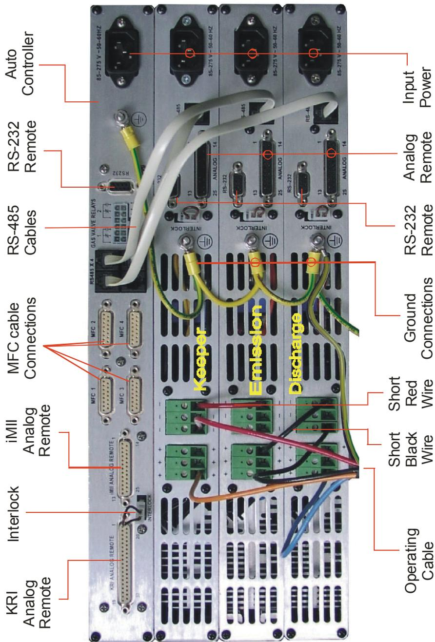
Figure 3-2. Rear view of controller for End-Hall ion source.
