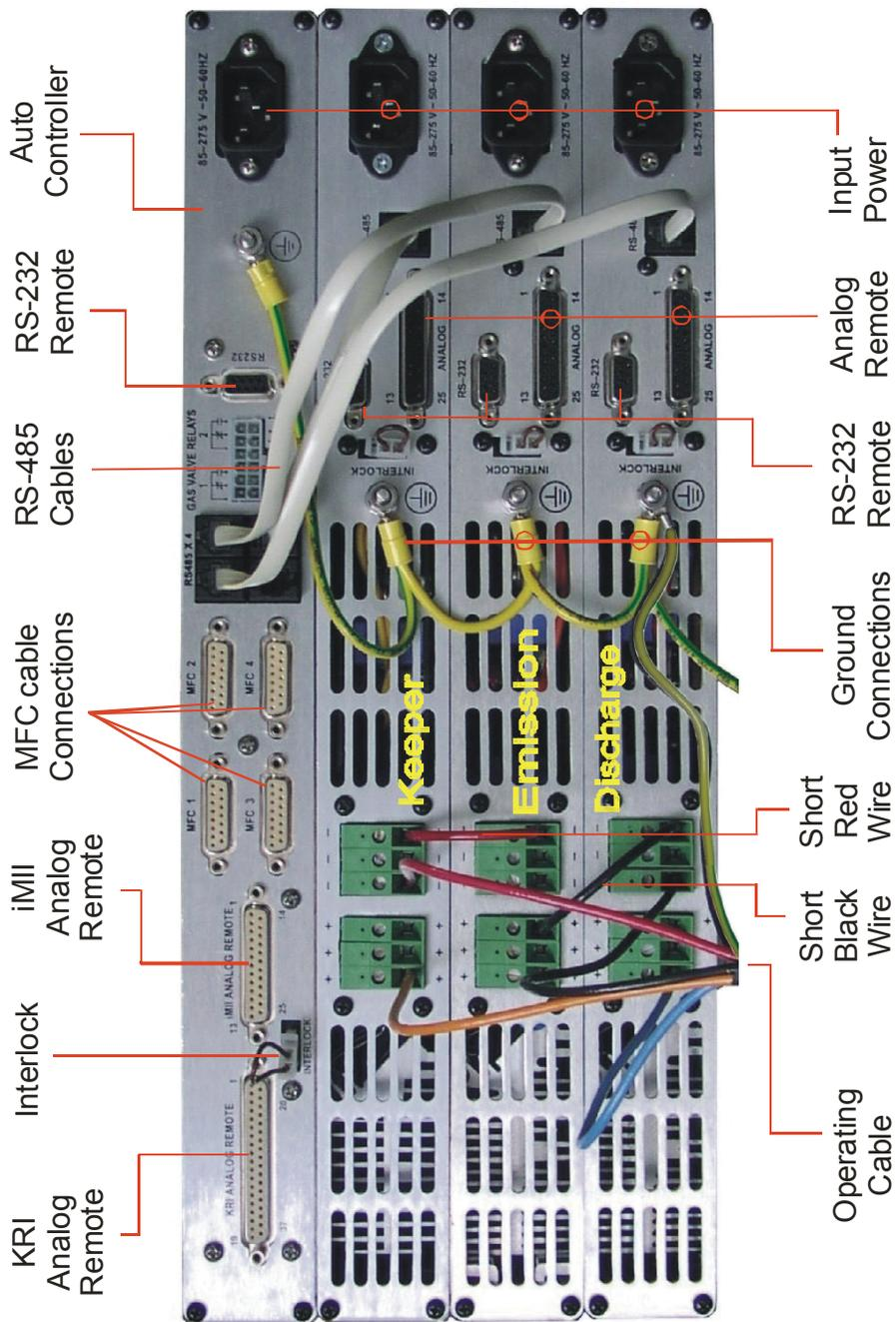
Figure 2-2. Rear view of controller for End Hall ion source.
