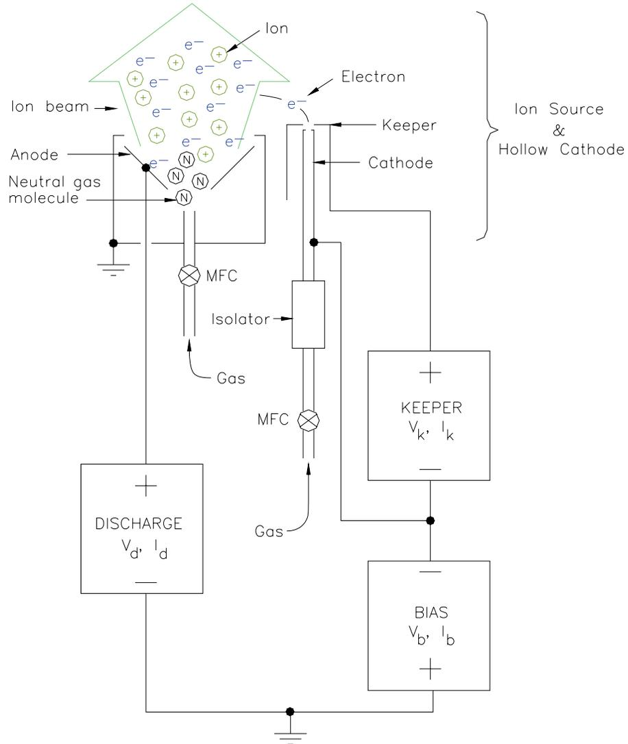
Figure 5-1. Schematic block diagram of ion source and power supplies.
