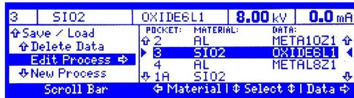
The material name of the real pocket can be changed by pressing the right joystick **R** to the left. The data set allocated to the virtual pocket can be selected from a list of stored data sets by pressing the joystick to the right.
