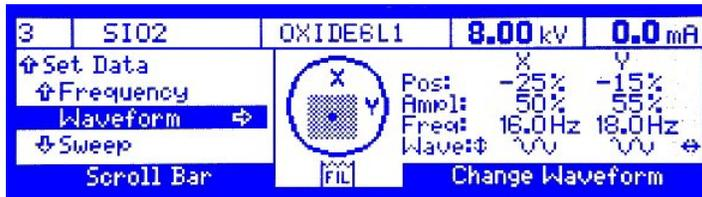
The functions can be selected with the right joystick. A wave symbol indicates the waveform that has been selected. In addition to the pre-set functions, the deflection forms can also be
