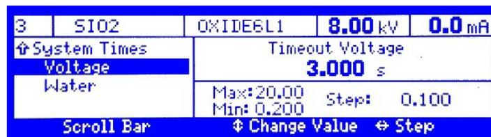
**Water** defines the duration in which a loss of the water flow on the evaporator results in a warning rather than an error. (the error would stop the process).
