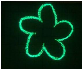
With  $f_p \gg f_c$  a propeller beam path is generated. The example on the left (sweep parameter = 15; center cold) shows a frequency ratio of  $f_p = 5 \times f_c$  meaning that the beam gravitates 5 times into its center during one revolution.
