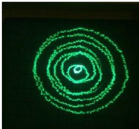
In the example above the pulsation frequency  $f_p$  would equal 2 Hz. With  $f_p < f_c$  a spiral beam path is generated. While the beam makes 30 revolutions (per second) it gravitates 2 times into its center. With a sweep parameter set to 15 (center hot) the thermal power input is concentrated to the center.
