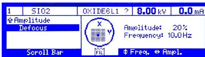
For all sweep modes a so called dynamic defocus can be applied. This mode superimposes a circle of the defocus frequency  $f_d$  with an amplitude  $A_d$  onto any beam path. The defocus amplitude  $A_d$  can be increased to a maximum
