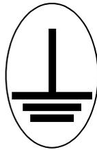
This symbol indicates where the protective earth ground is connected inside the instrument. Never unscrew or loosen this connection.
