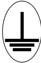
**This symbol indicates where the protective earth ground is connected inside the instrument. Never unscrew or loosen this connection.**
