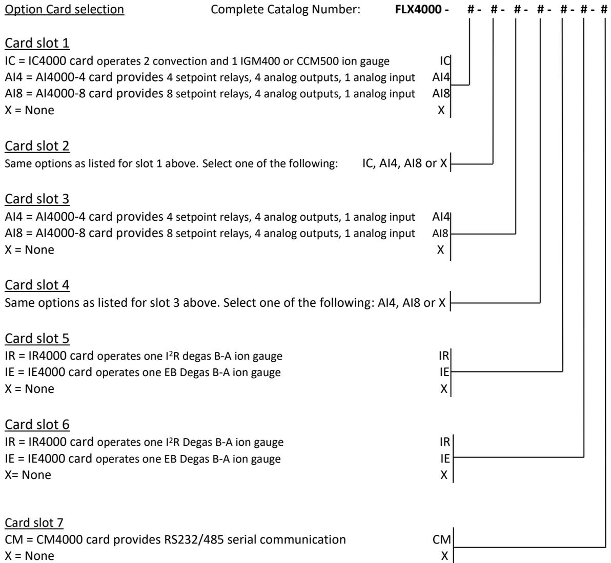
\* Maximum of two IC (IC4000) and two AI4 (AI4000-4) or AI8 (AI4000-8) option cards per FlexRax controller is possible.
