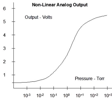
In general, one may use linear interpolation techniques to calculate the pressure using the non-linear analog output voltage measured at a specific pressure. You may also calculate the N<sub>2</sub>/air pressure represented by the non-linear analog output voltage for the original “S-curve” using a multi-segment, n<sup>th</sup> order polynomial function calculation listed on the following page.
