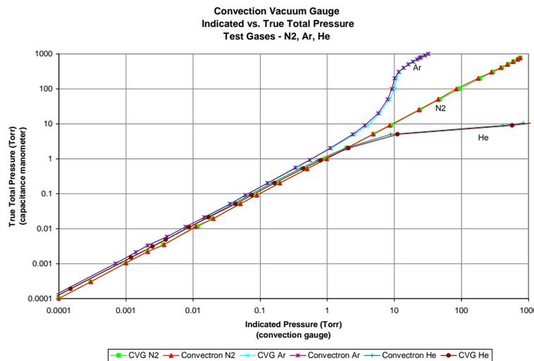
The Y-axis of the above chart is actual pressure as measured by a capacitance manometer, a diaphragm gauge that measures true total pressure independent of gas composition. The X-axis is the pressure reading indicated by the convection gauge under test. This chart shows readings for an InstruTech convection gauge (CVG) and Granville-Phillips® Convector® gauge to illustrate that the difference in the response for both of these types of gauges is virtually indistinguishable.
