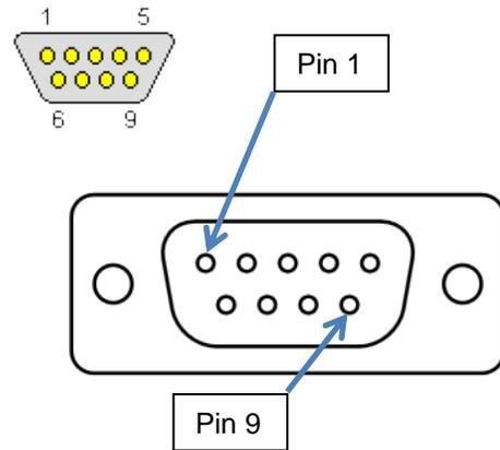
**Connect either RS232 or RS485 cable to *FlexRax* – DO NOT CONNECT BOTH AT THE SAME TIME**
