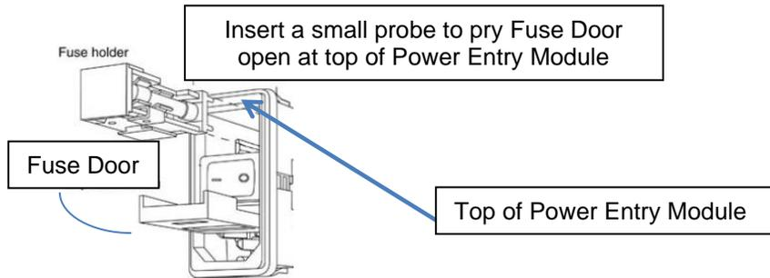
Using the small probe that you used to open the Fuse Door, gently pry the Fuse Holder away from the Power Entry Module (the Fuse Holder location is shown in the picture above).
