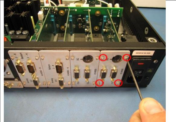
7. Slide the option card out of the enclosure. Add or replace card. When facing the back panel, always populate option cards from right to left. Do not leave empty slots between option cards.
