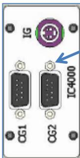
Connect the CVG101 *Worker Bee* cable(s) here. Connector(s) are labeled CG1 and CG2.
