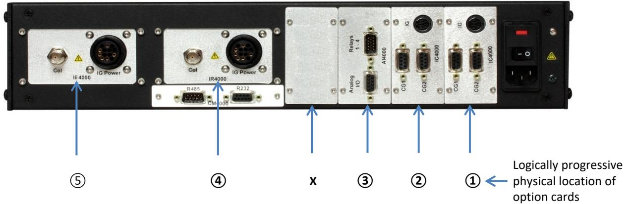
As discussed in the previous page, gauges and input/outputs are identified on the display with first number representing the physical location of the option card and the second number representing the number designation of the specific gauge or input/output on the option card as shown in the following example.
