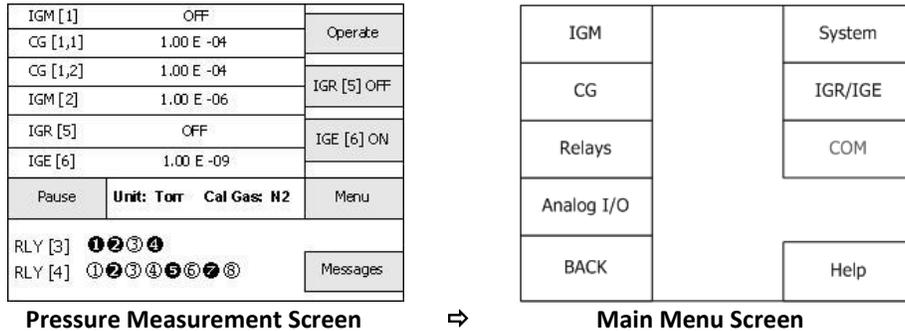
Press the **Relays** key in the Main Menu Screen above and the Relays Select Screen (or similar depending on option cards installed) will appear as shown below. Next, select any of the desired relays (for example **RLY [2,1]** ⇒ or **RLY [2,2]**, etc.) and the Relay Setup Screen for the selected relay will appear as shown below.
