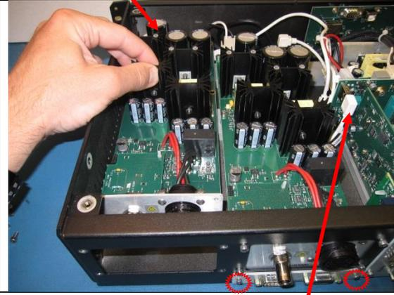
13. For the CM4000 option card, use a 3/82 in. Hex key to remove two socket head cap screws marked with red circles. Route the white cable connector attached to the CM4000 card under the IR4000 or IE4000 card as shown above.
