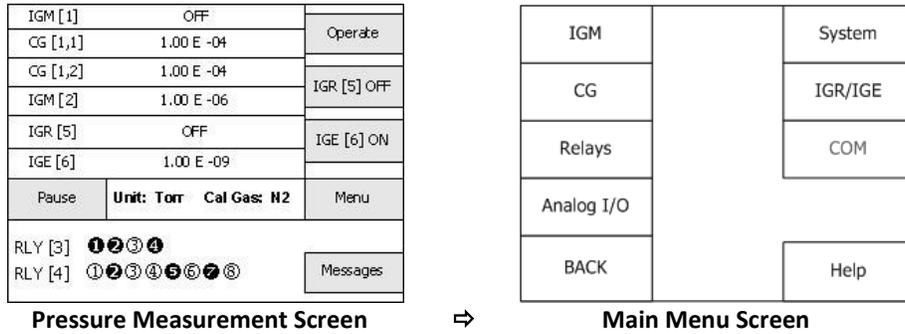
Press the **System** key in the Main Menu Screen above and the System Setup Screen appears as shown below.
