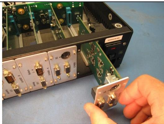
7. Remove four socket head cap screws marked with red circles in order to add or replace an Isection
