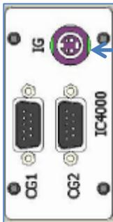
Connect the IGM400/CCM500 *Hornet* cable here. Connector is labeled IG.
