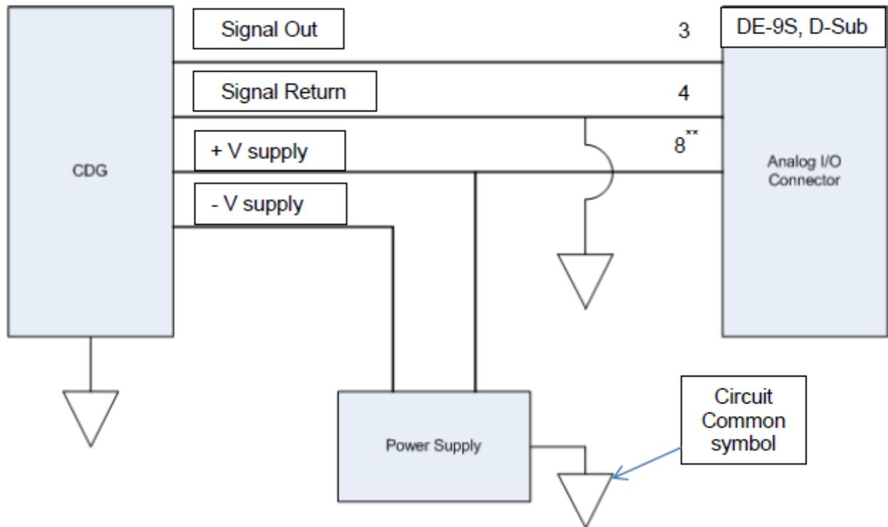
**\*\* Detection Requirement: Connecting Any Type of Device to the Analog Input**
