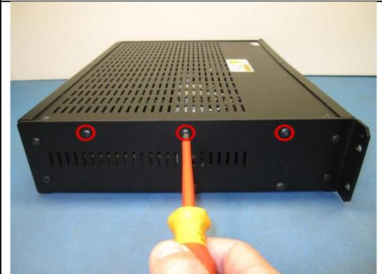
2. Remove all four screws of the top cover marked with red circles.
