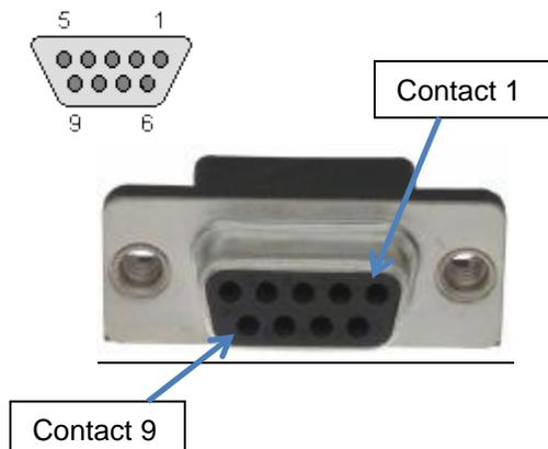
**Connect either RS232 or RS485 cable to *FlexRax* – DO NOT CONNECT BOTH AT THE SAME TIME**
