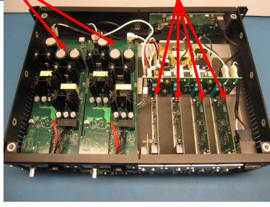
6. Remove four socket head cap screws marked with red circles in order to add or replace a specific IC4000 and/or AI4000 card (Use a 3/32 in. Hex key to remove screws).
