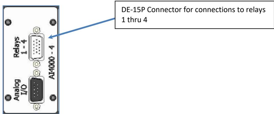
**15-pin (DE-15P) D-subminiature Relay Contactor Connections**
