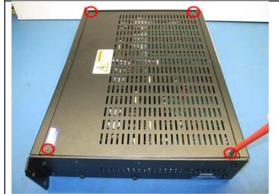
3. Slide forward top cover with a flat head screw driver inserted in slot shown below.
