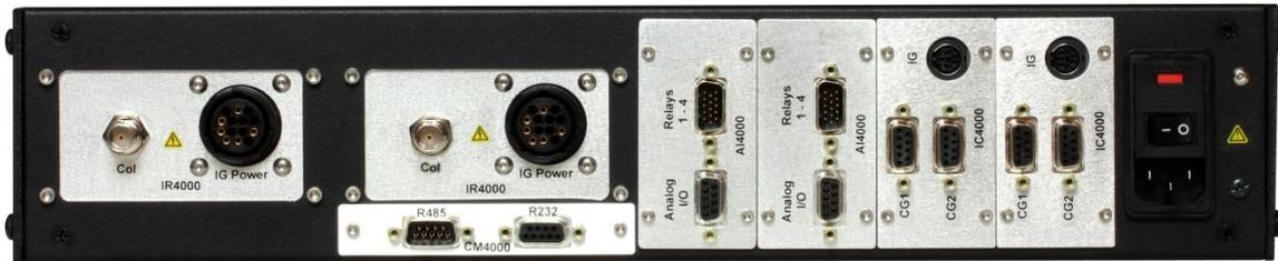
Option card labeled IR4000 operates a resistive degas, sometimes referred to as I<sup>2</sup>R Degas, hot filament nude or glass-enclosed B-A ion gauge (IG - InstruTech BA602/BA603 or similar).
