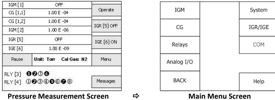
**Note** - If the CVG101 cable is not connected, the displayed key for that CG may be shown on display as “grayed-out”. CVG101 cable must be connected to allow programming of the CG menu.
