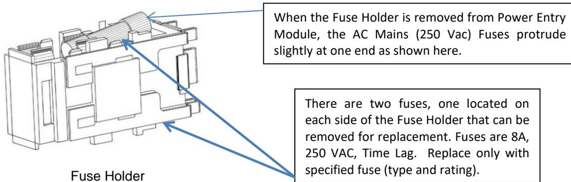
You will notice that the NEMA 5-15P/IEC 60321-1 C14 Power Cord must be disconnected from the *FlexRax* before you will be allowed to open the door that covers the access to remove the fuse holder. The two fuses protrude slightly from the fuse holder when the fuse is removed from the Power Entry module. This is by design to ensure that the end of the fuse makes contact with the terminals inside the module when the fuse holder is inserted.
