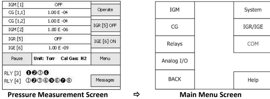
Press the **COM** key in the Main Menu Screen above and the COM Setup Screen will appear as shown below.
