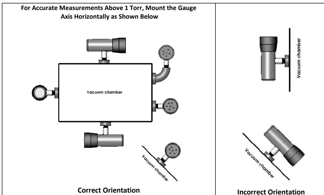
Mount the CVG101 with port down, if possible, to help minimize the effect of any particles or condensation from collecting in the gauge. Do not mount the CVG101 where it will be subjected to excessive vibration. Vibrations may cause unstable readings, measurement errors and possible mechanical stress to components in the CVG101.
