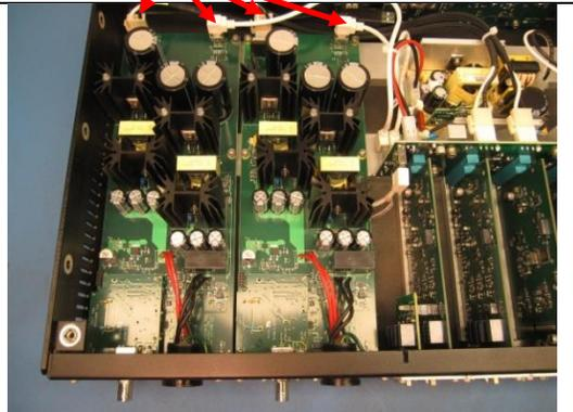
10. Disconnect both connectors attached to the IR4000 / IE4000 card.
