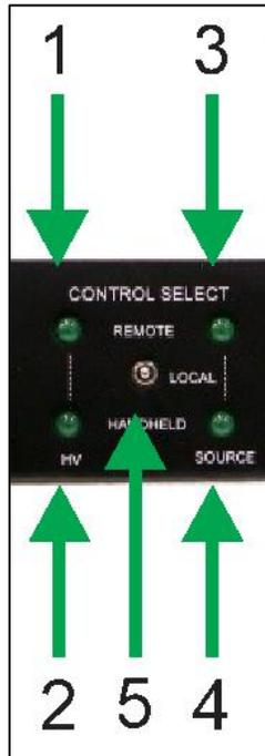
**Figure 4-5, Control Select Functions**
