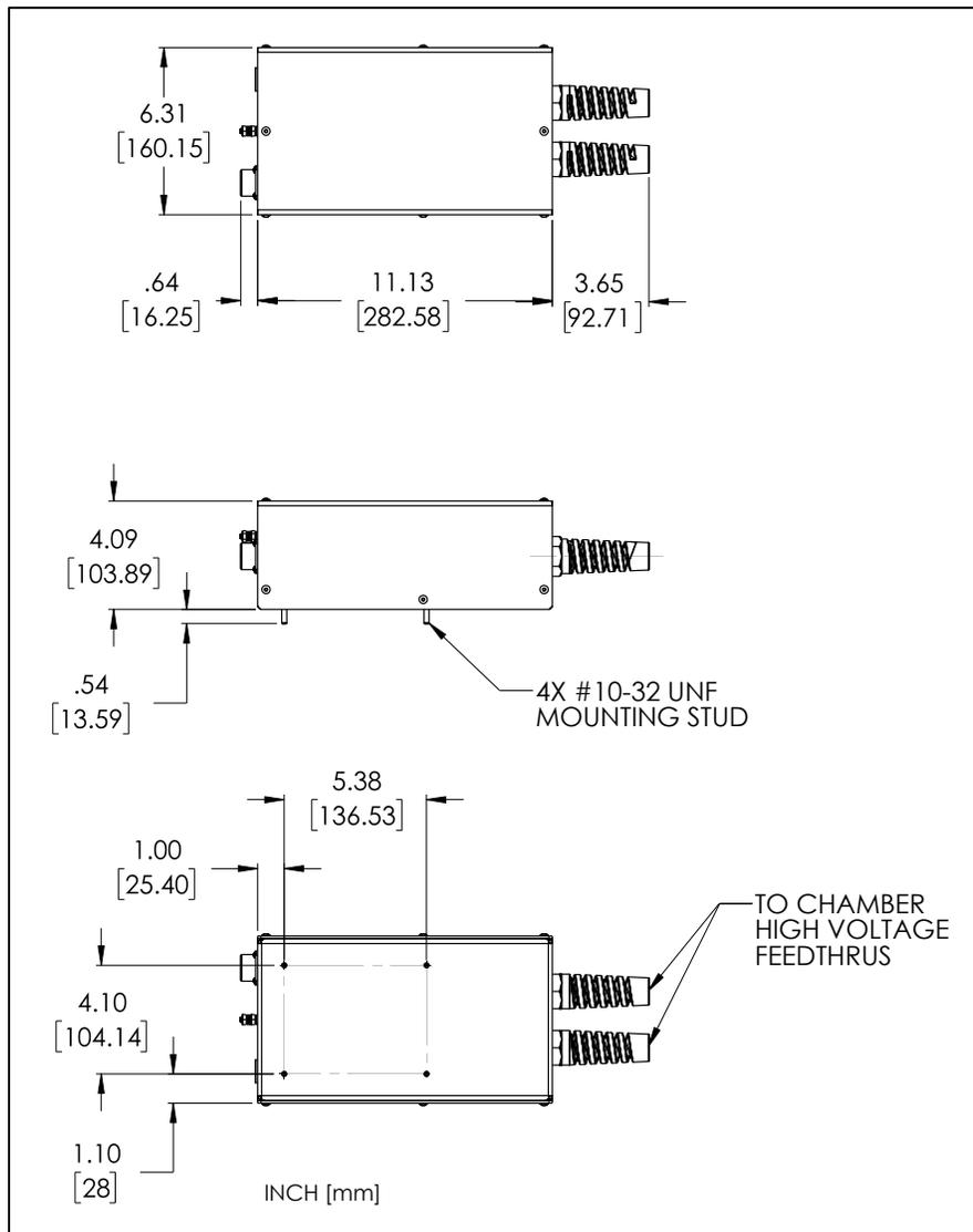
**Figure 2-3, ST Filament Transformer Dimensions**
