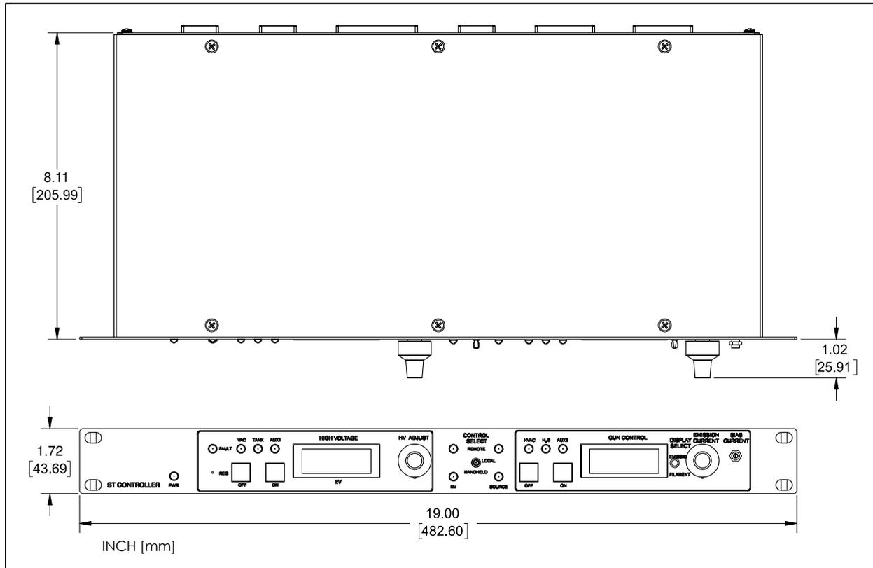
**Figure 2-4, ST Controller Dimensions**
