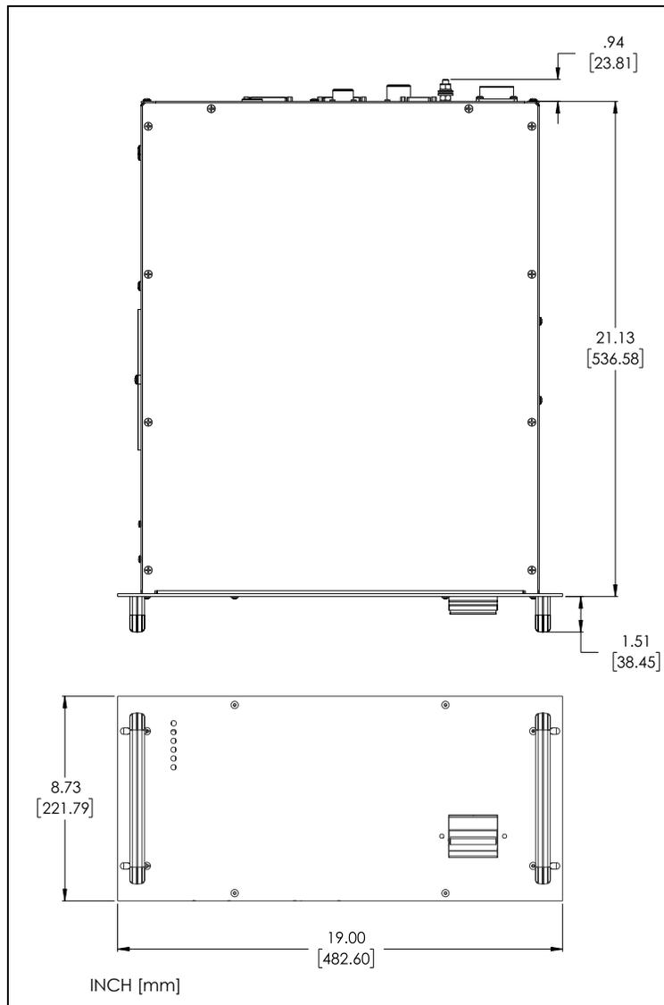
**Figure 2-2, ST HVPS Reference Dimensions**
