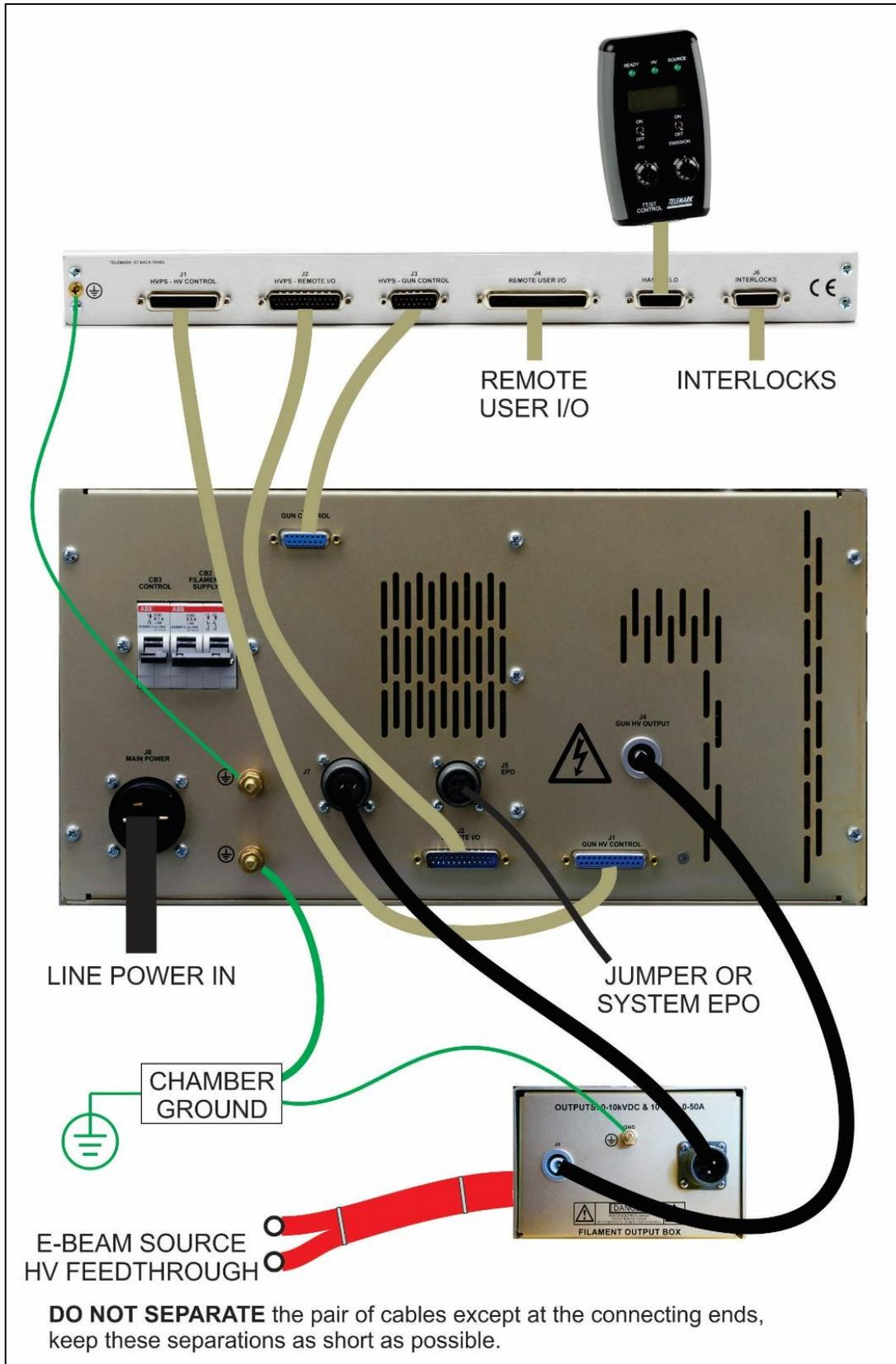
Figure 3-5, Interconnections for the ST Power Supply
