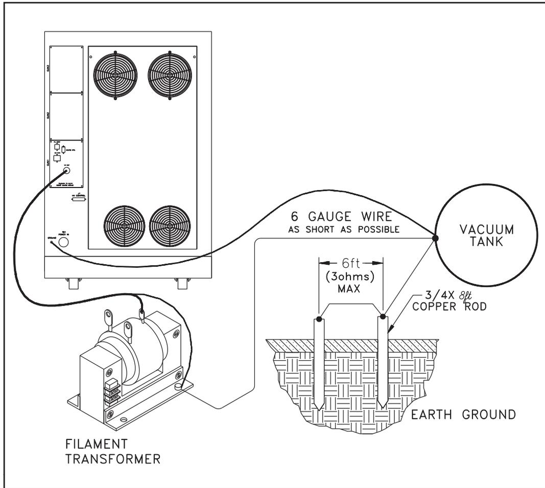
**NOTE - THE POWER SUPPLY MUST BE CONNECTED TO AN ISOLATED EARTH GROUND AS SHOWN IN FIG. 3-A AND 3-B, FAILURE TO CONNECT THE POWER SUPPLY TO AN ISOLATED EARTH GROUND COULD CAUSE SEVERE DAMAGE TO THE POWER SUPPLY AND/OR AUXILIARY ELECTRONIC CONTROL EQUIPMENT AND WILL VOID THE WARRANTY.**
