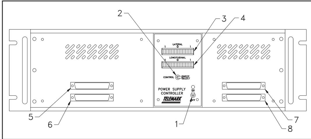
**3 & 4** POSITION L.E.D.s—show the relative position of the beam (in two axis—Lateral [left & right] and Longitudinal [near & far]) in the pocket.
