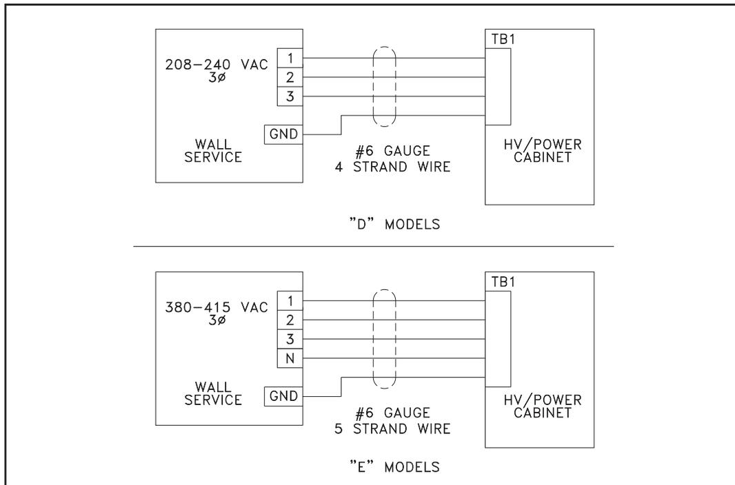
Figure 3-F HV/Power Cabinet Connections
