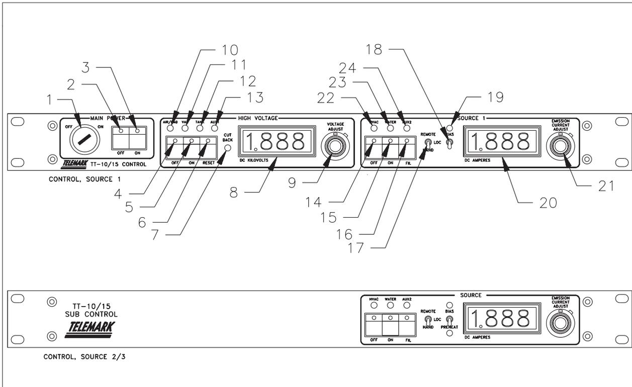
The state of the High Voltage interlocks is continuously checked. If any condition is not correct, the corresponding indicator will not be lit. The High Voltage Indicator lights are (left to right):
