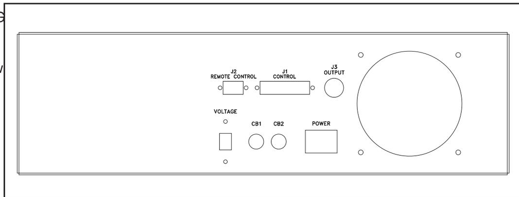
This Sweep allows the customer to select the input-voltage range, with a switch (on the back panel) for running on either 105—120 VAC or 208—240VAC. Switched to the lower range, it can plug into domestic wall outlets, ~115VAC.
