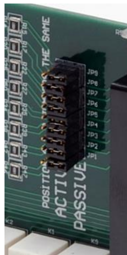
Figure 3-16, 37-Pin I/O Card, Active/Passive Jumpers
